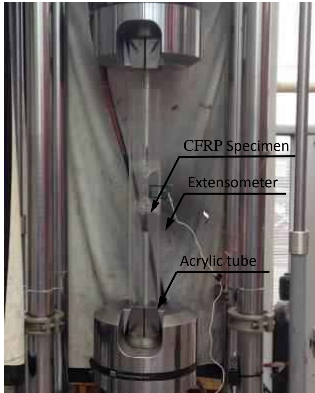
Figure 3.10: Tensile test of CFRP specimen at NCSU
