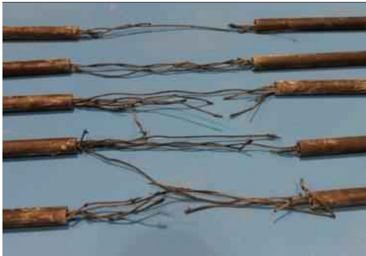
Figure 3.7: Typical mode of failure of CFRP tension specimens (Sherbrooke University)
