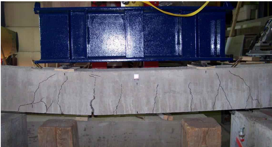
Figure 4.55: Crack pattern of the control beam specimens
