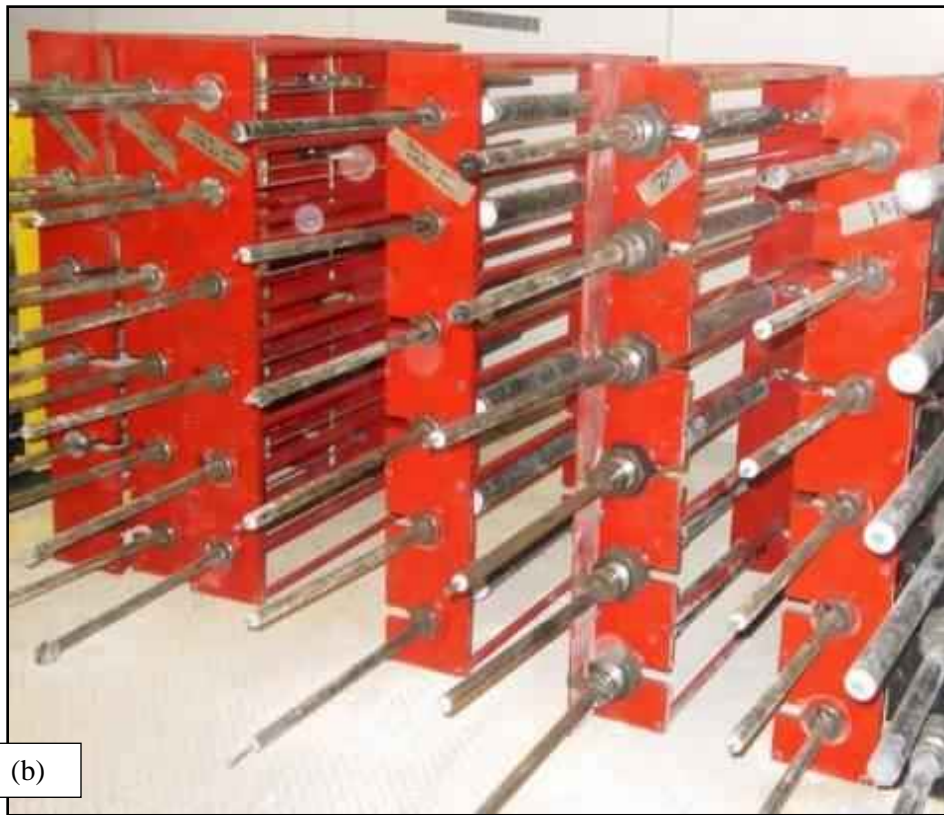
Figure 3.16: Sustained creep load frame during fixing the CFRP specimens with and without alkaline solution: (a) T=22^{\circ}\text{C} [72]; (b) T=60^{\circ}\text{C} [140 ^{\circ}\text{C} ]
