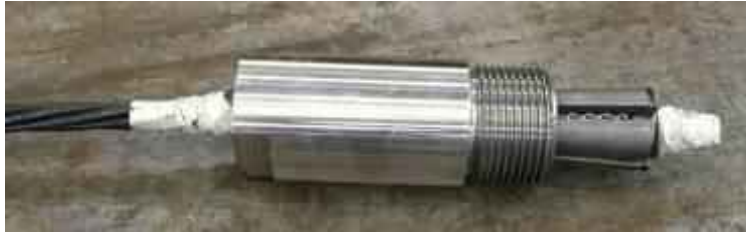
(i) Sleeve with wedges pressed inside it
