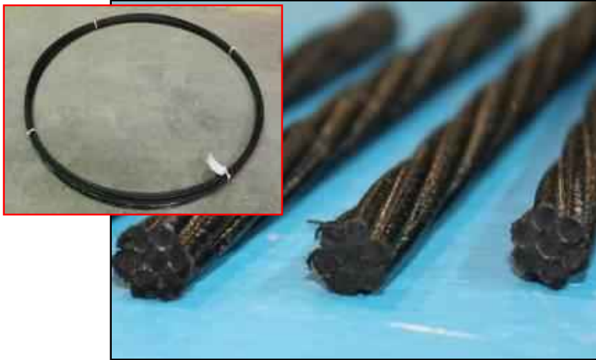
Figure 2.13: (a) Overview of cross-section of 7.5 mm CFRP tendon specimens; (b) CFRP cable as received (Benmokrane et al. 2016)
