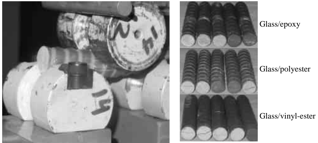
Figure 4.31: Setup for short-beam testing and typical failure mode
