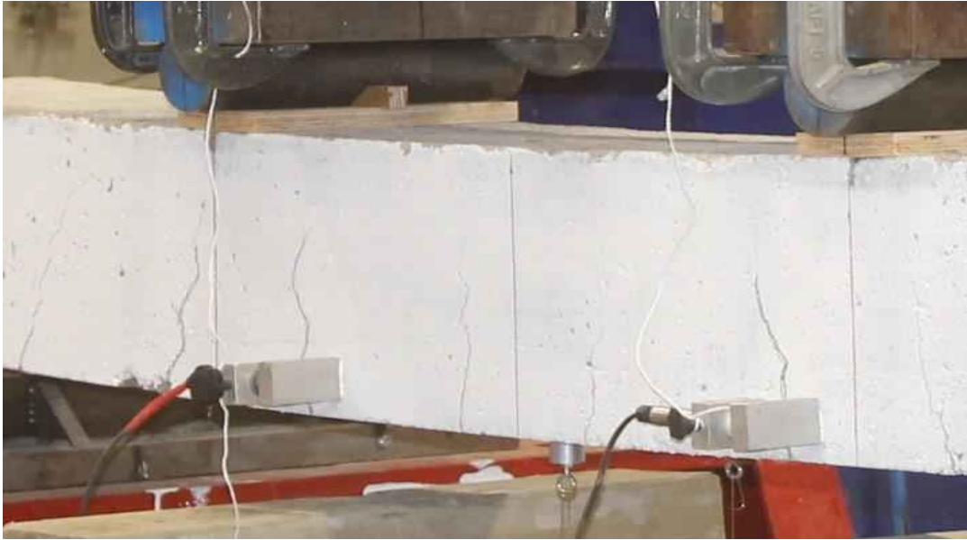
Figure 4.54: Crack pattern of the conditioned beam specimens
