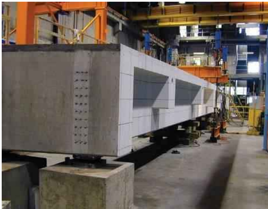
Figure 2.22: Test setup for flexural loading of DT girder (Grace et al. 2003).
