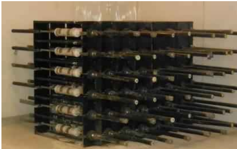
(b) GFRP specimens (with load=30%) in environmental chamber at 60°C [140°F]
