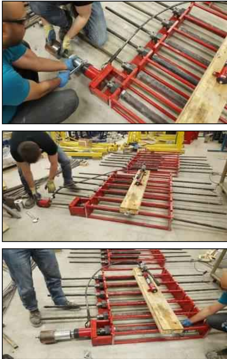
Figure 3.15: Steel frame used to subject CFRP tendons to sustained load
