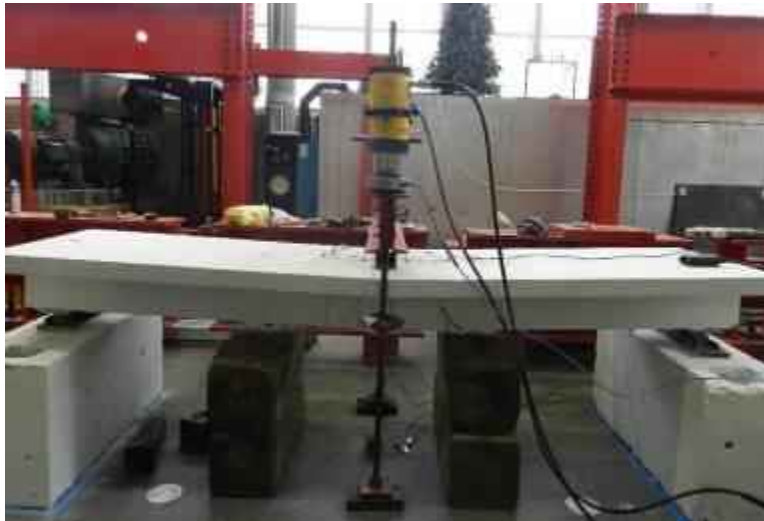
Figure 6.15: Failure of control beam#1
