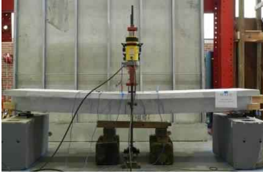
Figure 6.20: Failure of beam#4 after 3 months of exposure (Bottom Beam).
