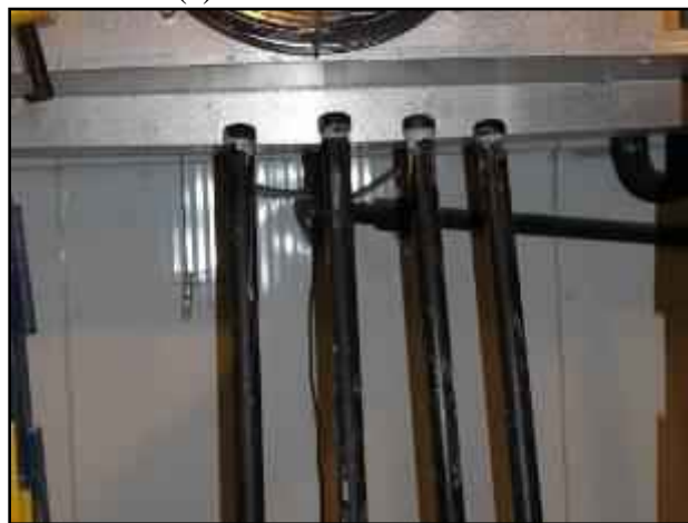
(b) PVC tubes included CFRP specimens and filled with alkaline solution inside the chamber
