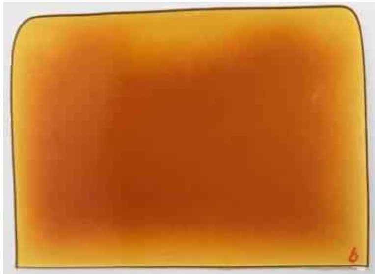
Figure 5.15: Inconsistency of epoxy resin within the same plate.
