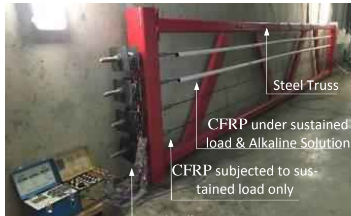
Figure 3.20: Steel truss with 4 tensioned CFRP tendons
