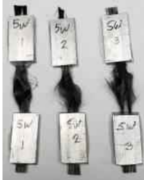
Figure 5.5: Typical carbon fiber specimens after testing.
