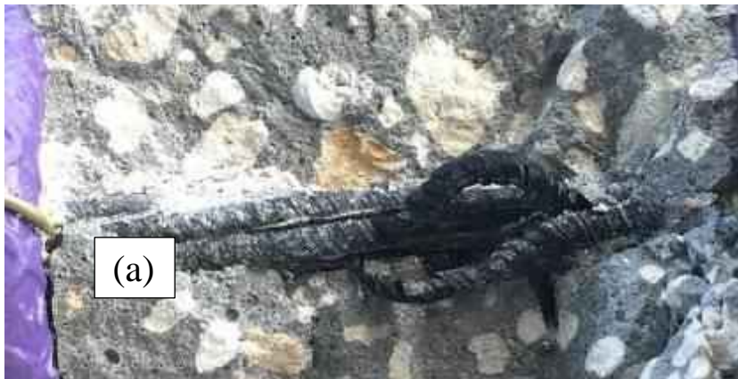
Figure 6.28: Failure of beam#8 after 12 months of exposure (Bottom Beam).
