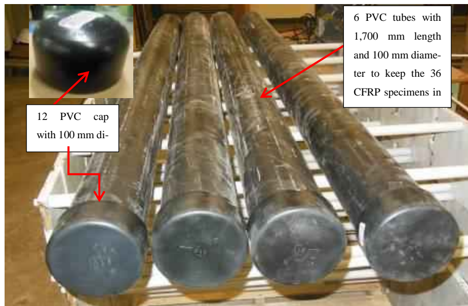
Figure 3.12: The CFRP specimens exposed to alkaline solution inside PVC tubes
