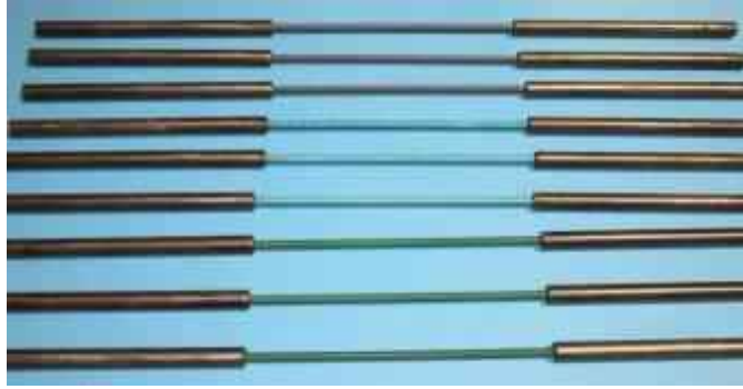
Figure 4.15: Typical test GFRP specimens
