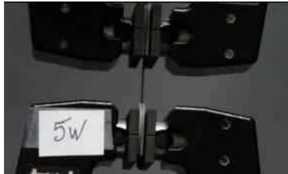
Figure 5.4: Tensile testing of carbon fibers specimen.
