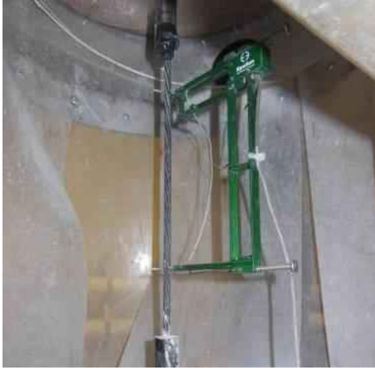
Figure 3.6: Typical tensile test setup at Sherbrooke University
