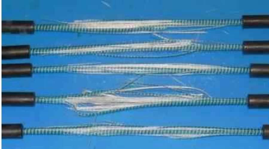
Figure 4.25: Typical mode of failure of isopolyester GFRP bars
