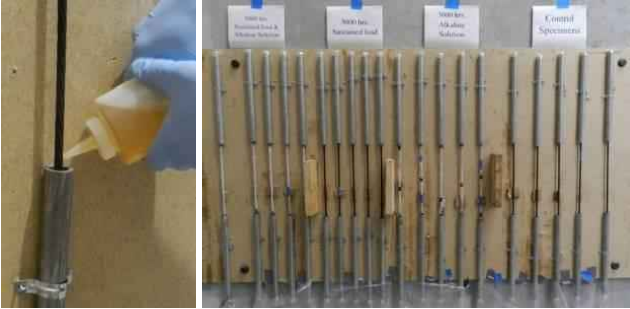
Figure 3.9: Preparation and curing of anchorages at NCSU
