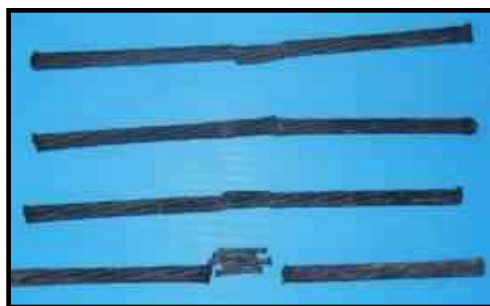
Figure 3.32: Typical shear failure of CFRP specimens
