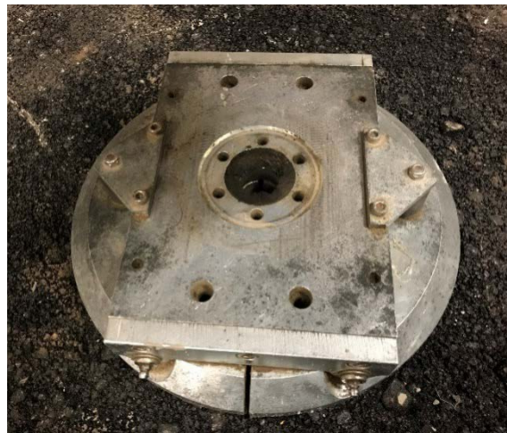
Figure 7-29. Top view of the FWD loading plate used for dynamic loading.
