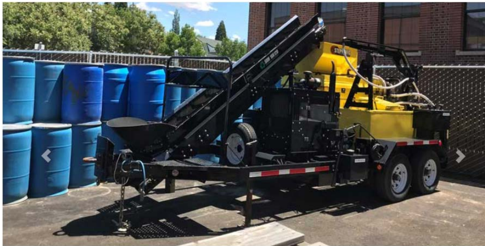
Figure 7-27. Half-ton asphalt mixer used to mix and produce PMA and HP AC mixes for PaveBox .
