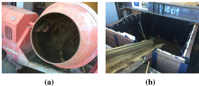
Figure 7-23. SG deposition: (a) soil mixing in the mechanical mixer, and (b) placement of moist soil in PaveBox.
