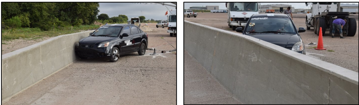
Figure 6.1. Transition and Test Vehicle Geometrics for Test No. 469689-2-1.
