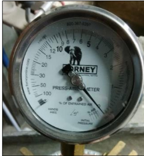
(a) Air meter reading zero with full water during calibration
