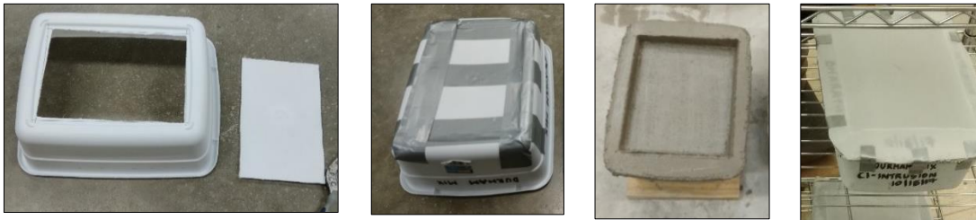
Figure 3.10. Slab preparation and ponding
