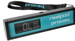
Figure 3.9. Resipod used for SR measurement
