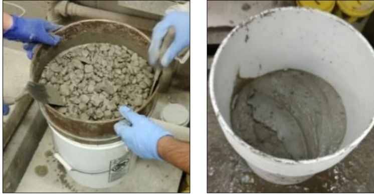
Figure 3.2. Sieving concrete using the #4 sieve (left) to obtain the mortar (right)
