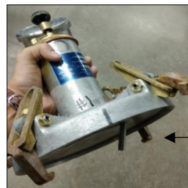
(b) Shortened calibration tube attached to the air meter
