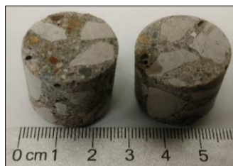
Figure 3.8. Concrete plugs used for MIP analysis
