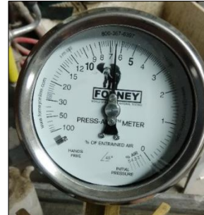
(c) Air meter reading 6.5% after removing 429.5 g water during calibration
