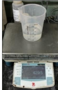
(b) Water removed (429.5 g) during calibration
