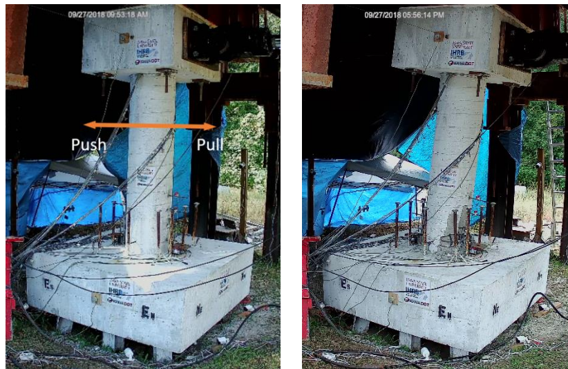
Figure 5.40. Column drift at the end of Phase I (left) and Phase II (right)
