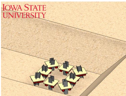
3. Plywood sealing the pile sockets
