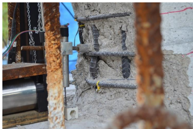
Figure 5.42. Buckling of longitudinal reinforcing bar
