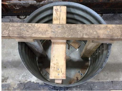
Figure 5.11. Plywood for closing the CSP with CSP hanger
