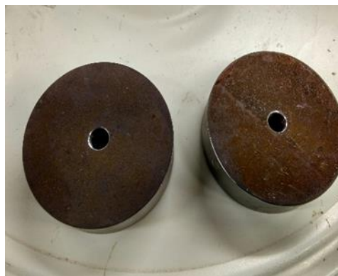
Figure D.2. Iron disks for holding the rod
