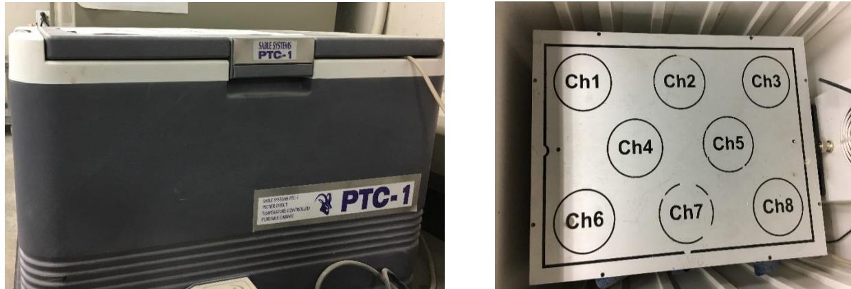
Figure 3.2. Isothermal calorimeter (left) and channels for holding samples (right)
