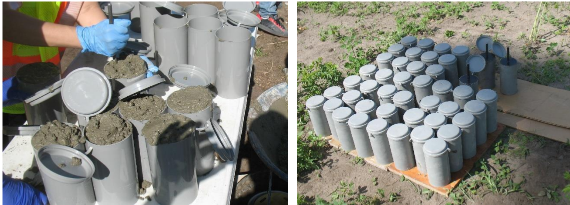
Figure 5.12. Casting cylindrical specimens (left) and curing specimens in field conditions at the job site (right)
