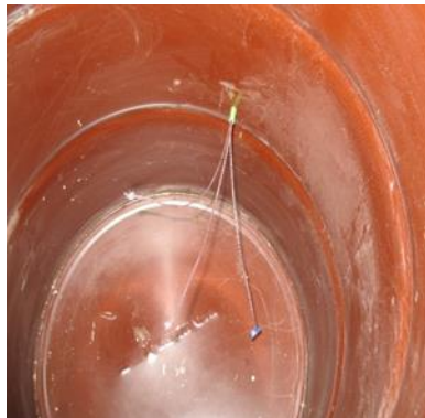
Figure B.2. Thermocouple wires through drilled hole
