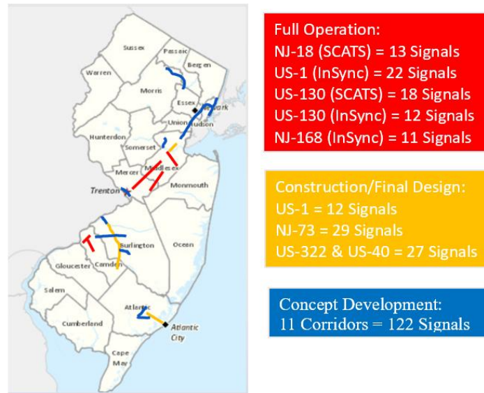
Figure 19. NJDOT Adaptive Traffic Signal Control (ATSC) system, 2019 (Red: In Full Operation; Yellow: In Construction and Final Design; Blue: concept Development)
