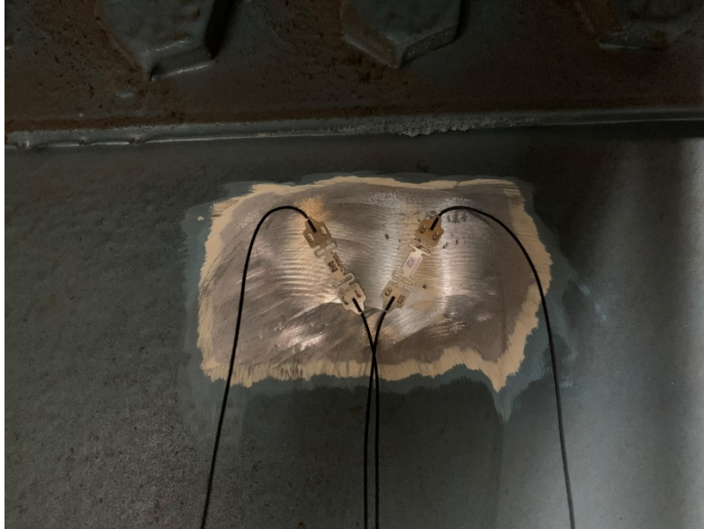
Figure 24 Typical rosette gage installation
