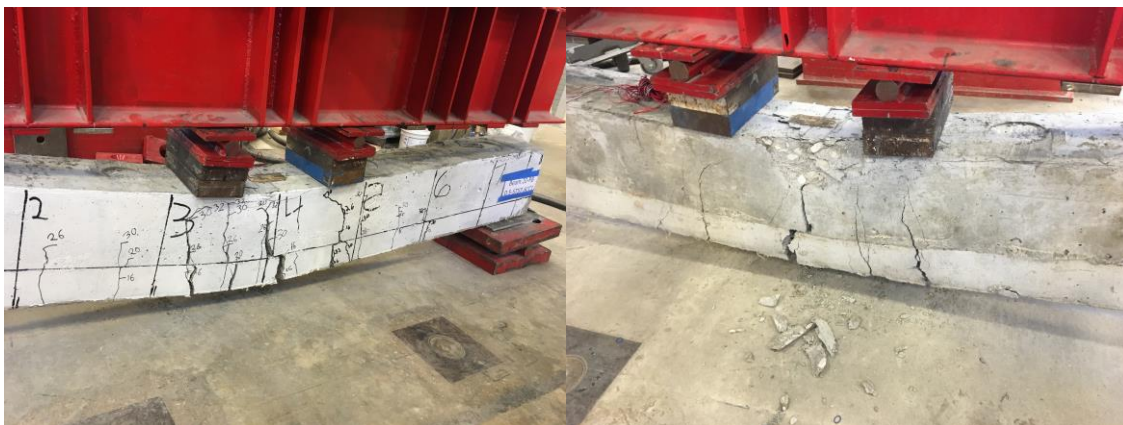
Figure 5-13: Testing of Repaired beams
