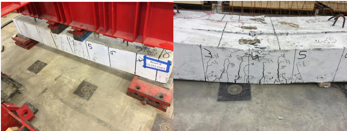
Figure 5-12: Testing of monolithic beams
