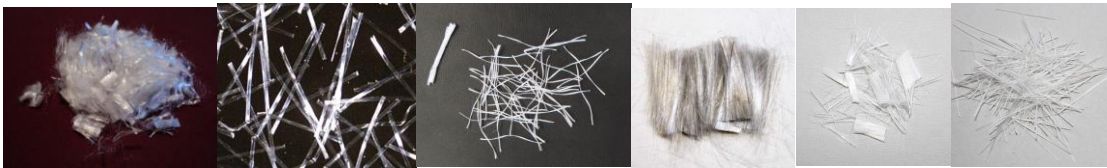
Figure 2-8: Different types of syntactic fibers; polypropylene micro, polypropylene macro, polypropylene macro strand, nylon micro, poly (from left to right)
