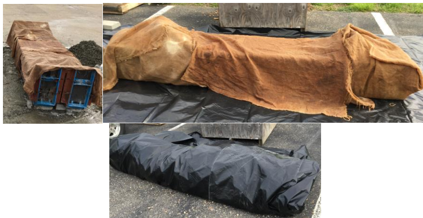
Figure 5-6: Curing of the beams and cylinder specimens using wet burlaps
