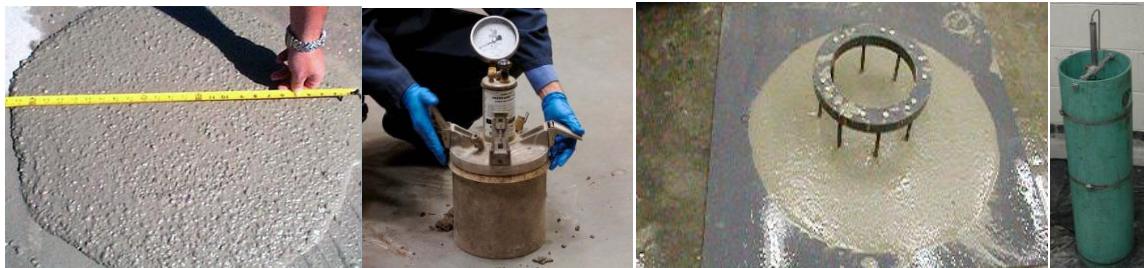
Figure 3-1: Testing fresh properties
