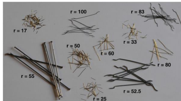
Figure 2-28: Different fibers tested [37]
