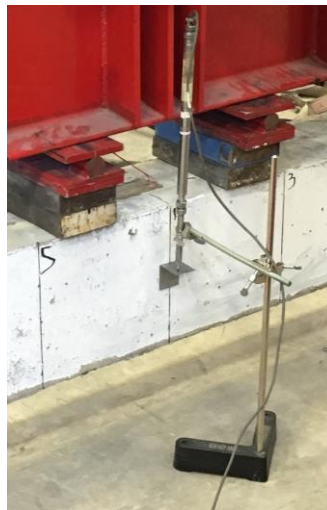
Figure 5-5: LVDT to monitor deflection of the beam
