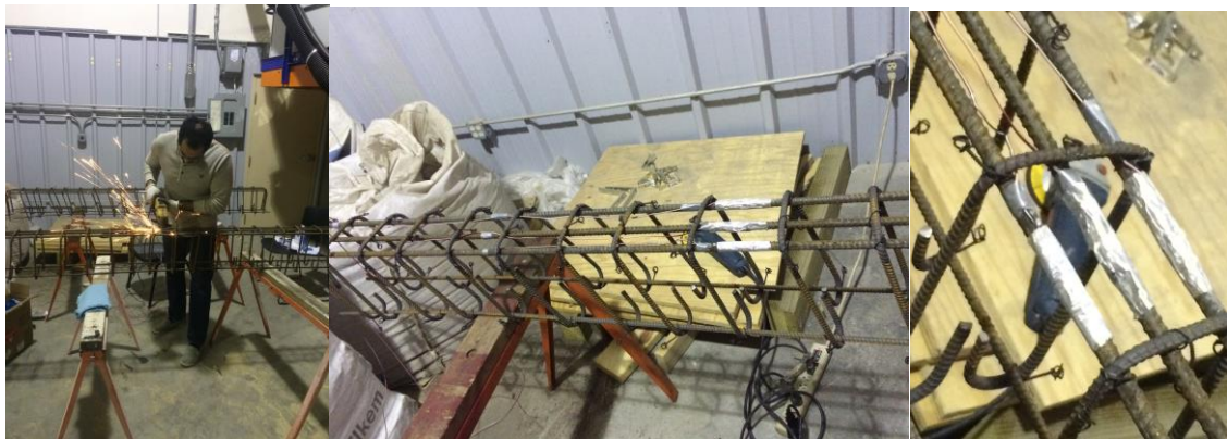
Figure 5-3: Attaching of the strain gages to steel rebar
