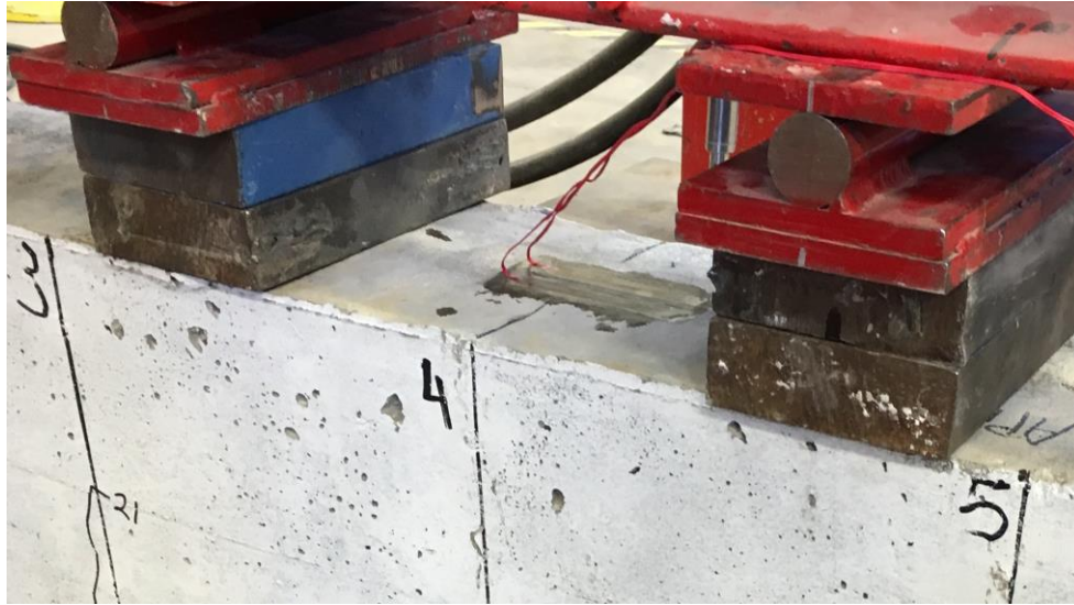
Figure 5-4: Concrete surface attached strain gages
