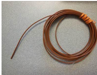
Figure 2 - Thermocouple used for concrete temperature measurement
