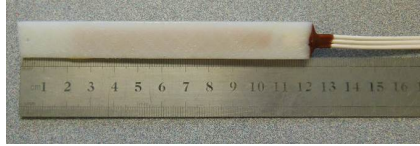
Figure 1 - Embedded strain gauge for monitoring shrinkage deformation
