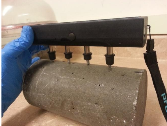
Figure 34- Surface resistivity measurement
