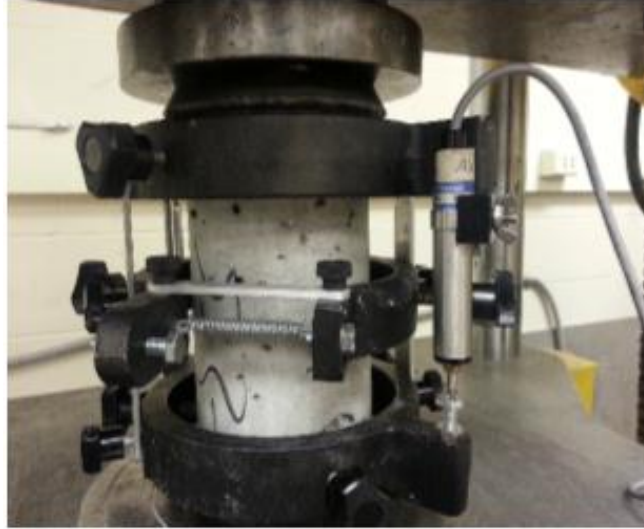
Figure 28- Modulus of elasticity test setup
