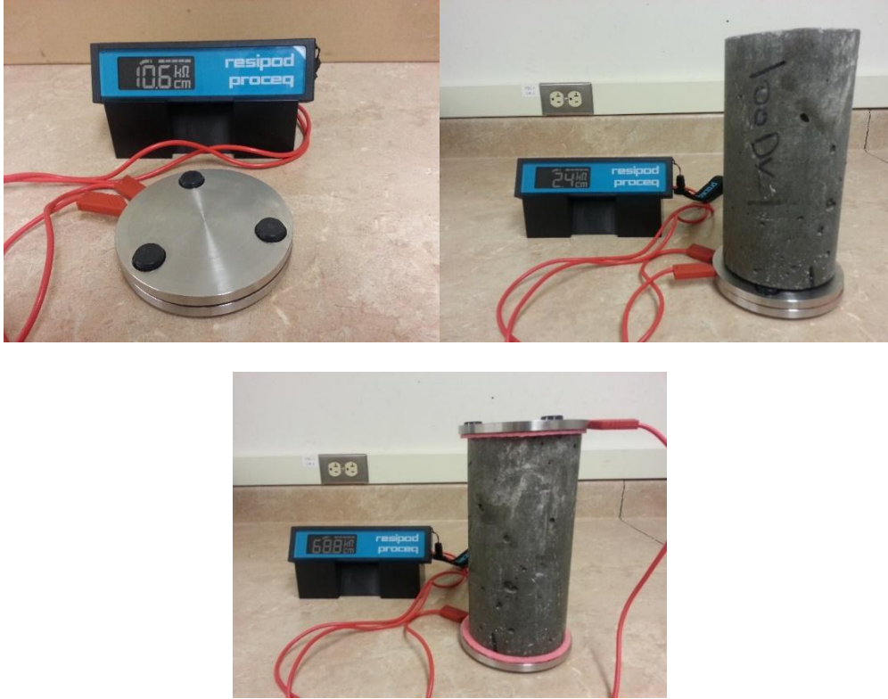
Figure 35- Measuring bulk electrical resistivity
