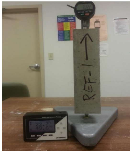
Figure 29- Length measurement for drying shrinkage
