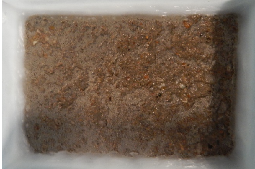
Figure 6-15. Control Specimen After 25 Cycles
