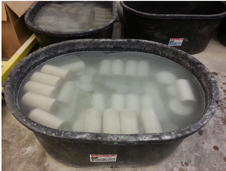
Figure 9-3. Constant Temperature Lime Water Tempering Tank
