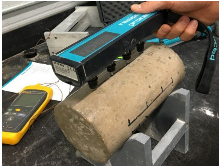
Figure 6-1. Surface Electrical Resistivity Test
