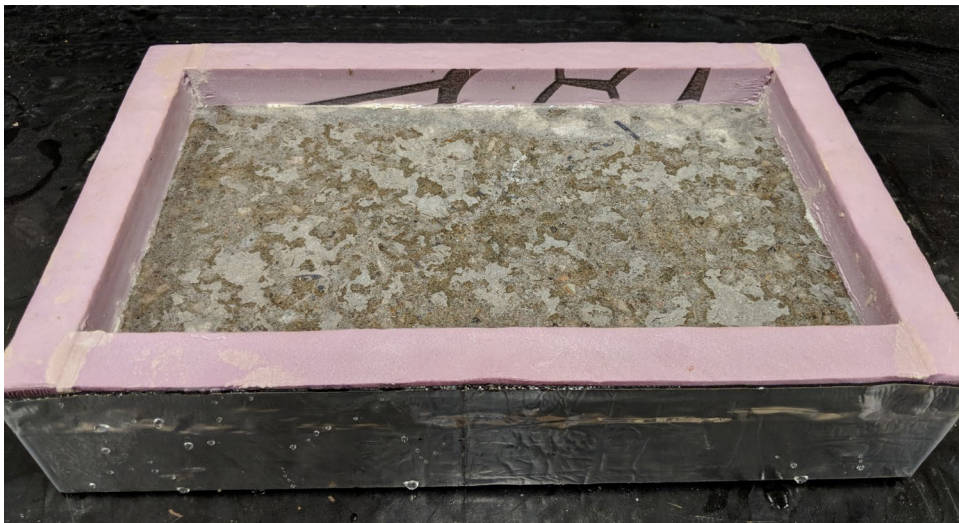
Figure 9-13. Mix 3-60 Salt Scaling Specimen at 50 Cycles
