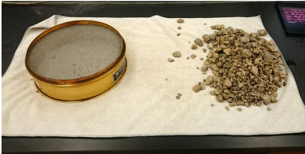
Figure 7-2. Aggregate Preparation for Moisture Measurements
