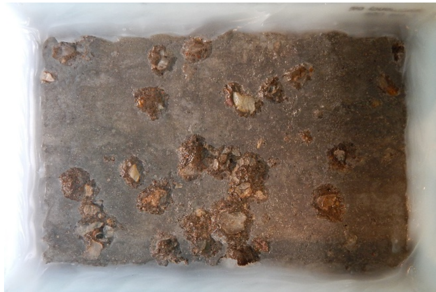
Figure 6-18. 75 Percent RCA Specimen After 50 Cycles
