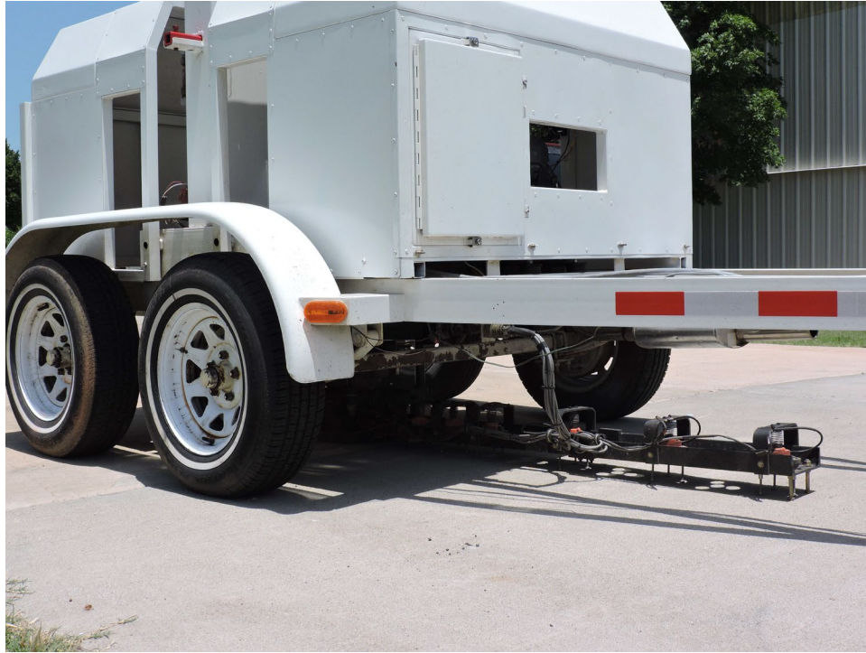
Figure 10-16. FWD Testing of Pavement Panels
