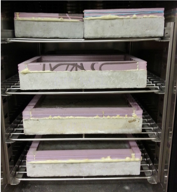
Figure 9-5. Salt Scaling Specimens within Environmental Chamber
