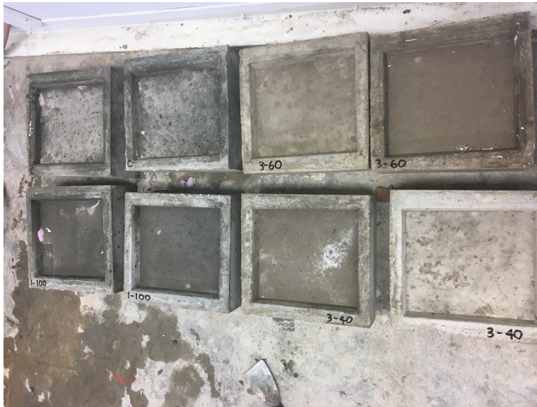
Figure 5-5. Salt Scaling Specimens Air Curing
