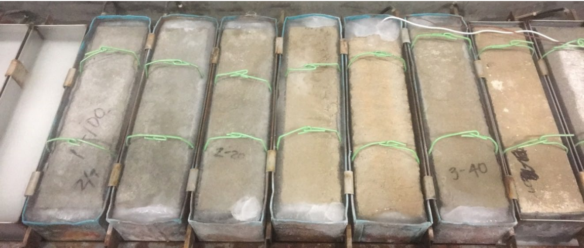
Figure 5-1. Freeze/Thaw Specimens within Test Chamber
