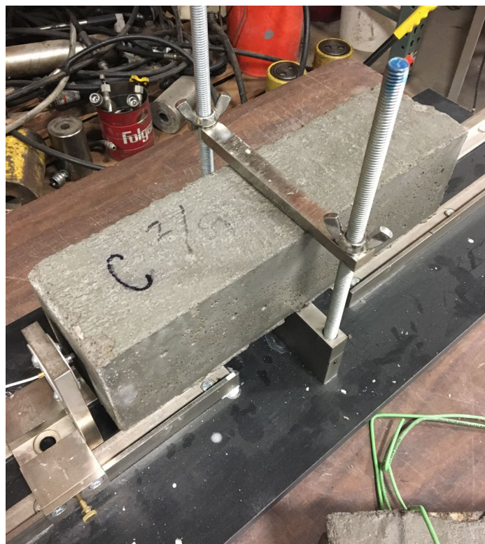
Figure 9-2. Longitudinal Dynamic Modulus of Elasticity Test Setup
