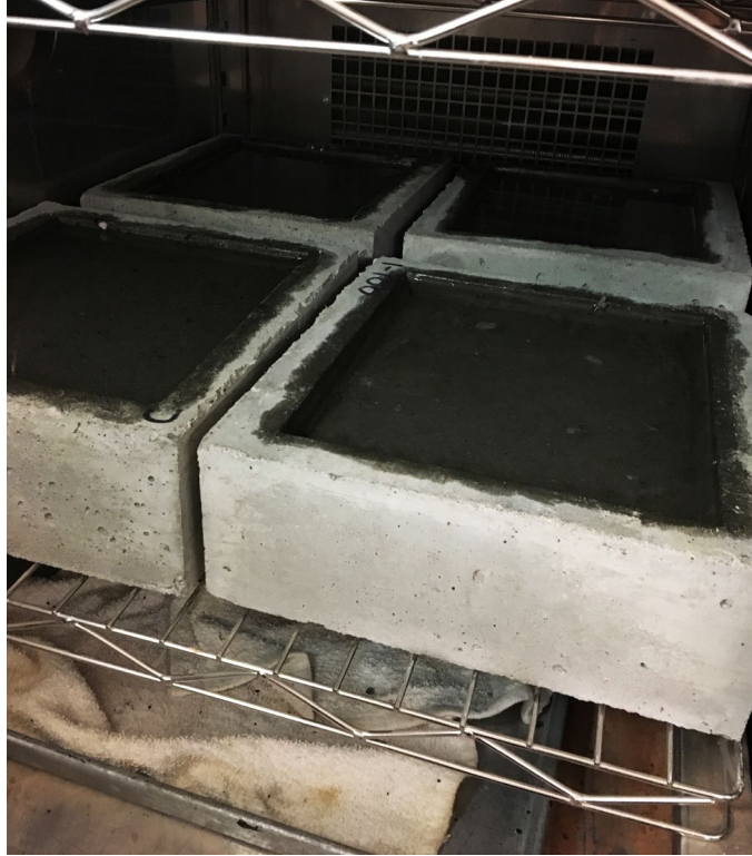
Figure 5-6. Salt Scaling Specimens within Environmental Chamber
