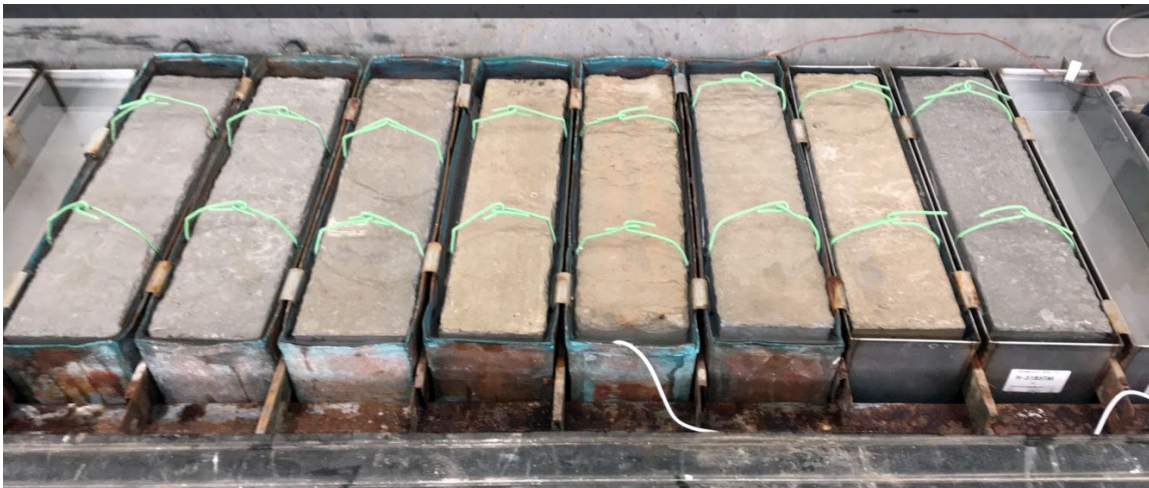
Figure 9-1. Freeze/Thaw Specimens within Test Chamber
