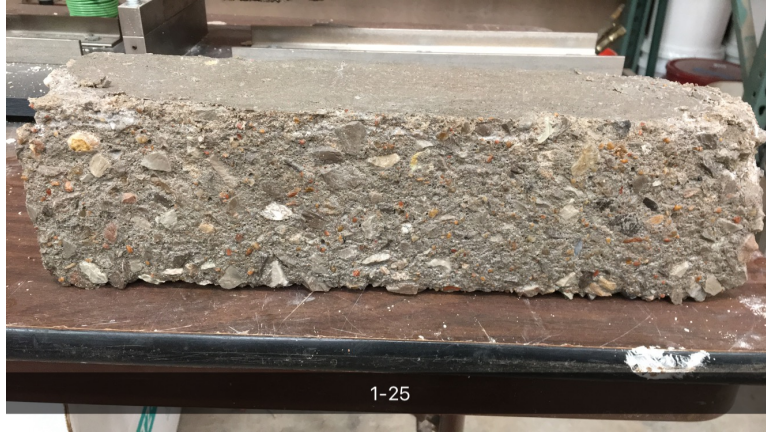
Figure 5-9. Mix 1-25 Specimen at 304 Freeze/Thaw Cycles
