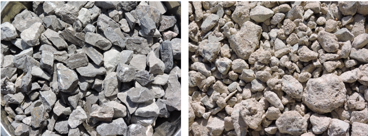
Figure 3-2. No. 57 Limestone (left) and Recycled Concrete Aggregate (right)
