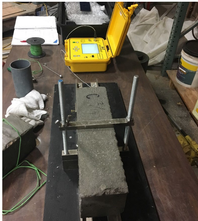
Figure 5-2. Longitudinal Dynamic Modulus of Elasticity Test Setup
