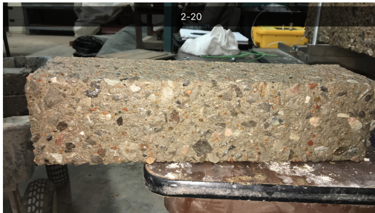
Figure 5-10. Mix 2-20 Specimen at 304 Freeze/Thaw Cycles
