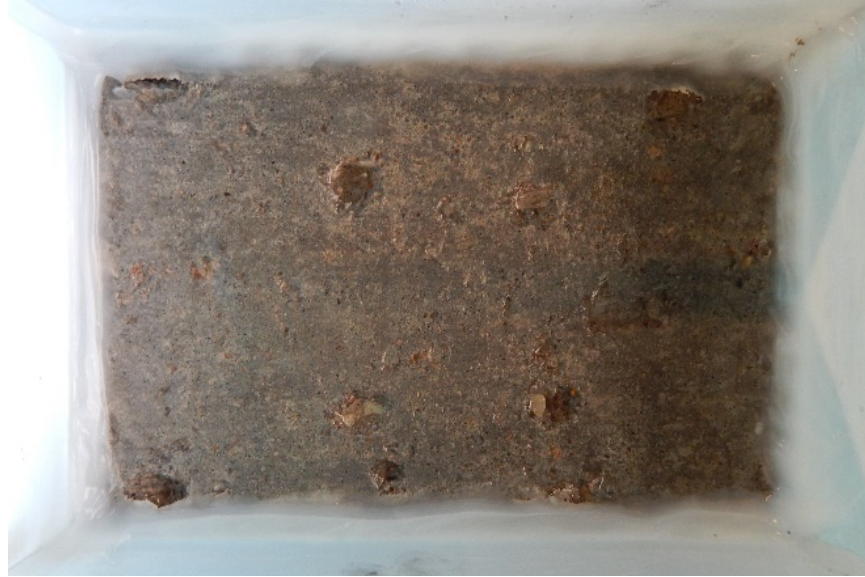
Figure 6-17. 50 Percent RCA Specimen After 50 Cycles
