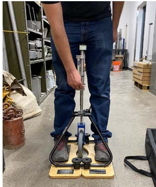
Figure 1 - BDRP indenter being lowered onto the surface to measure readings
