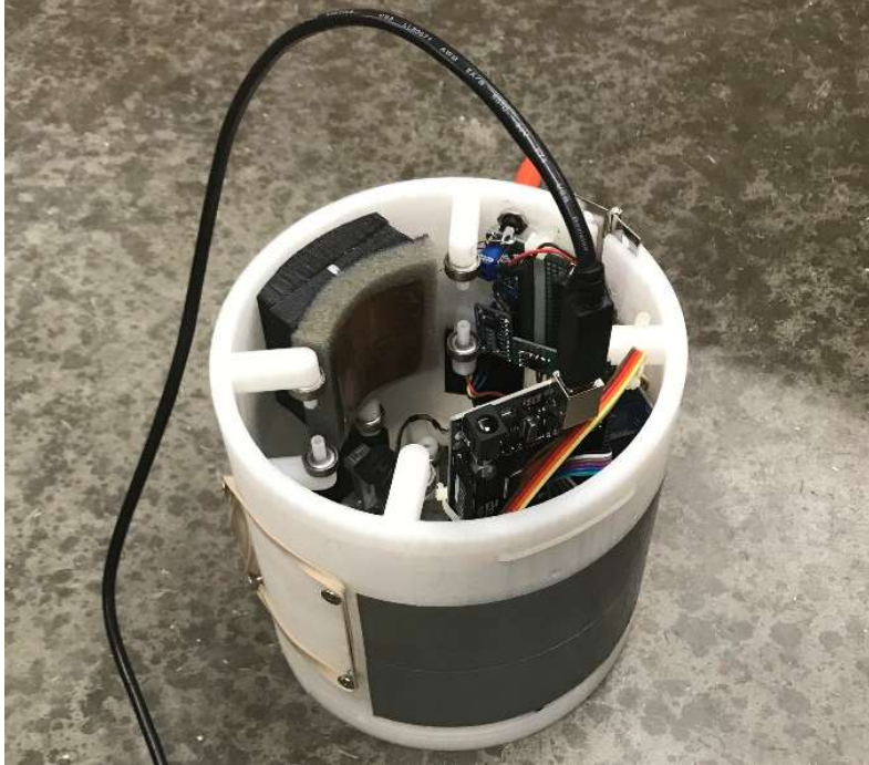
Figure 6.4 TIU-I placed in the vertical calibration position away from steel mass. Patent Pending.
