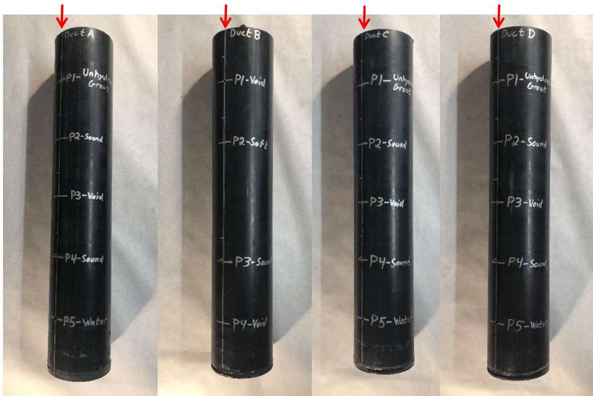
Figure 7.3 Side view of ducts A-D showing the locations of P1-P5 (different grout configurations). Arrows are keyed to positions shown in Figure 7.1
