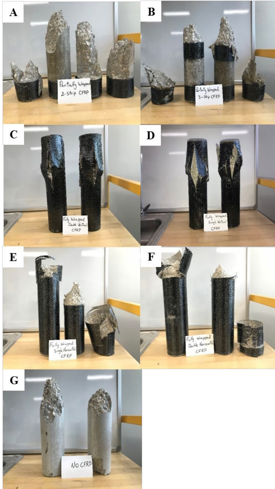
Fig. 5. Column specimens after axial loading. The specimen IDs are as follows: (a) CG1-1&2, (b) CG2-1&2, (c) CG3-1&2, (d) CG4-1&2, (e) CG5-1&2, (f) CG6-1&2, (g) CG7-1&2
