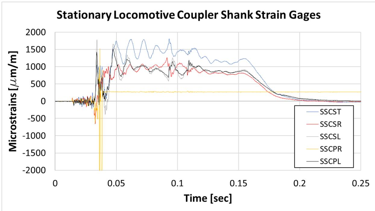
Figure 35. Stationary Locomotive Coupler Shank Strain Results
