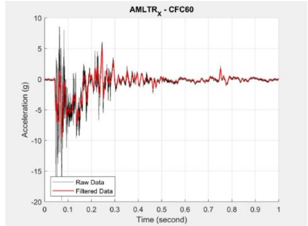
**Figure B8. AMLTR\_X Accelerometer Data**
