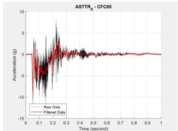
Figure B36. ASTTR\_X Accelerometer Data
