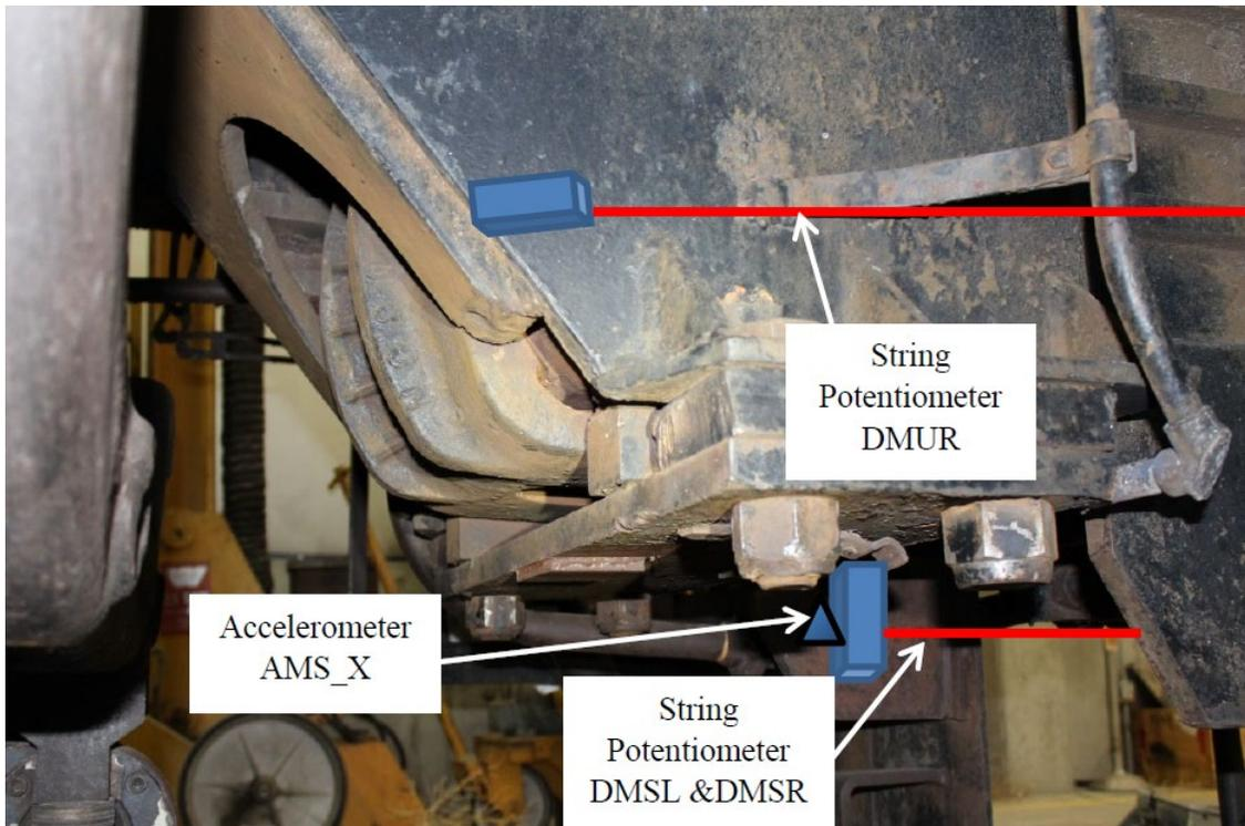
**Figure 9. Right Side Mobile Locomotive String Potentiometers**
