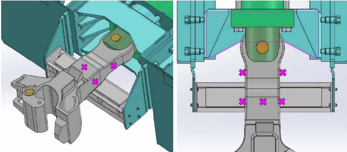
**Figure 22. Strain Gage Locations on Stationary Locomotive Coupler**
