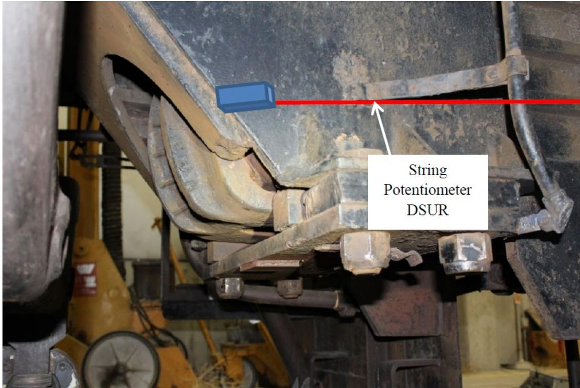
**Figure 21. Stationary Locomotive Underframe String Potentiometer Right**
