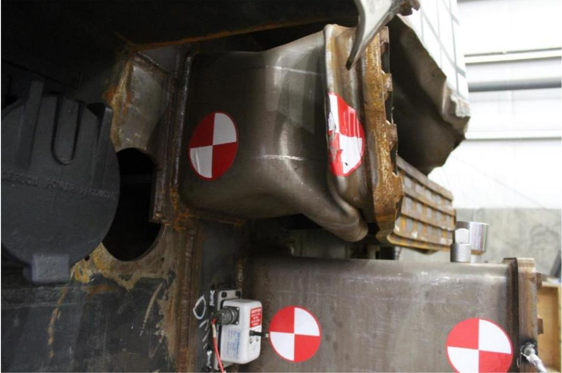
**Figure 40. Crushed Anti-climber**
