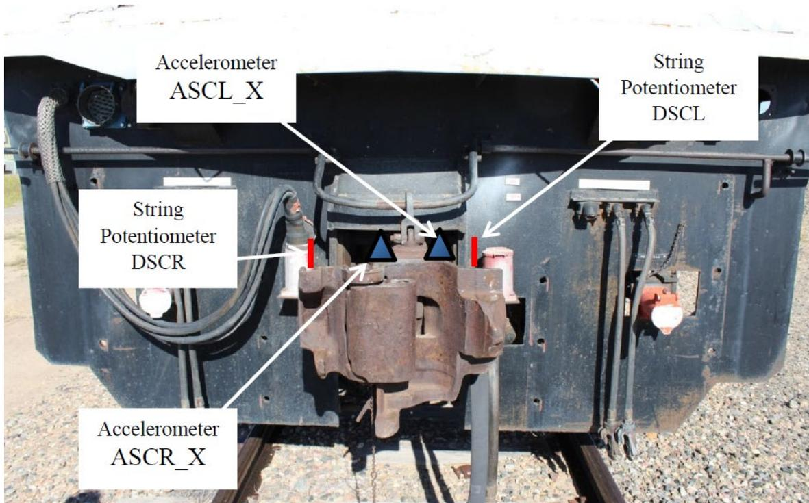
**Figure 19. Stationary Locomotive Coupler Instrumentation**
