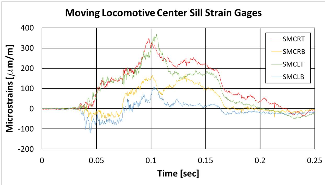
**Figure 33. Mobile Locomotive Center Sill Strain Results**
