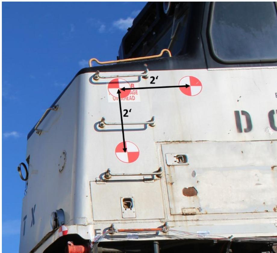
**Figure A2. Target Spacing for Locomotive 4117**
