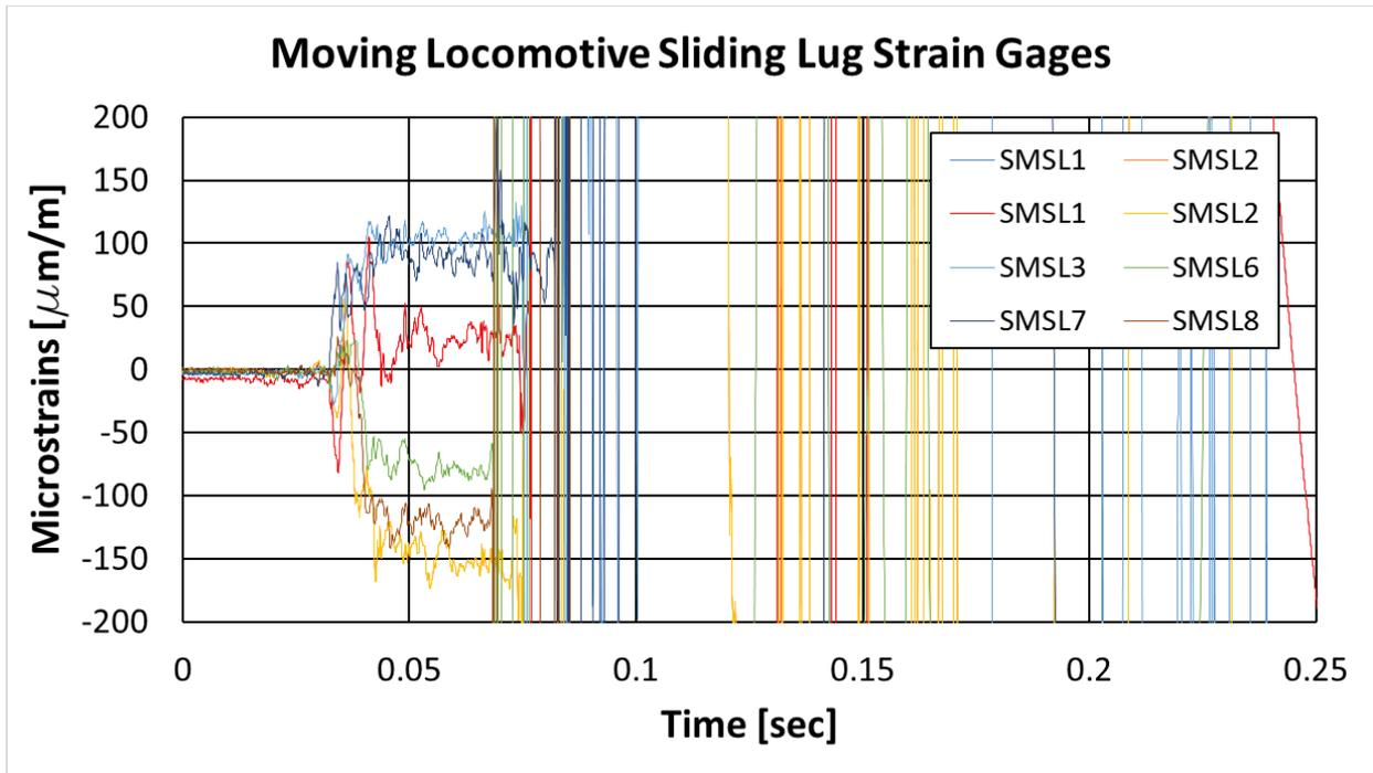
Figure 30. Mobile Locomotive Sliding Lug Strain Results
