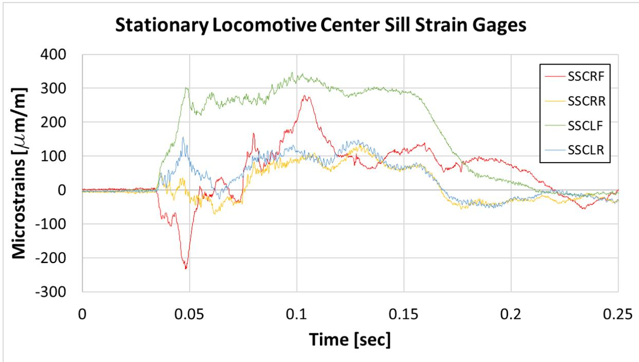
Figure 36. Stationary Locomotive Draft Sill Strain Results
