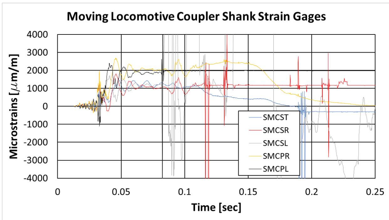
Figure 29. Mobile Locomotive Coupler Shank Strain Results
