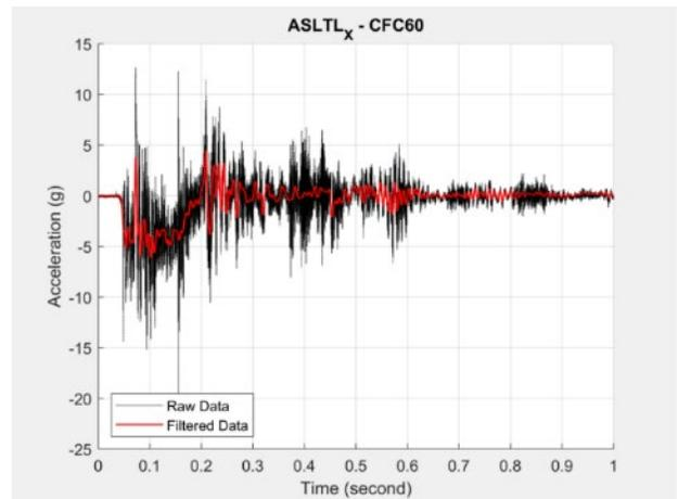
Figure B28. ASLTL\_X Accelerometer Data
