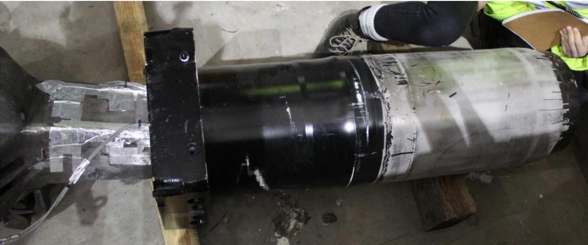
**Figure 41. Activated Push-Back Coupler**
