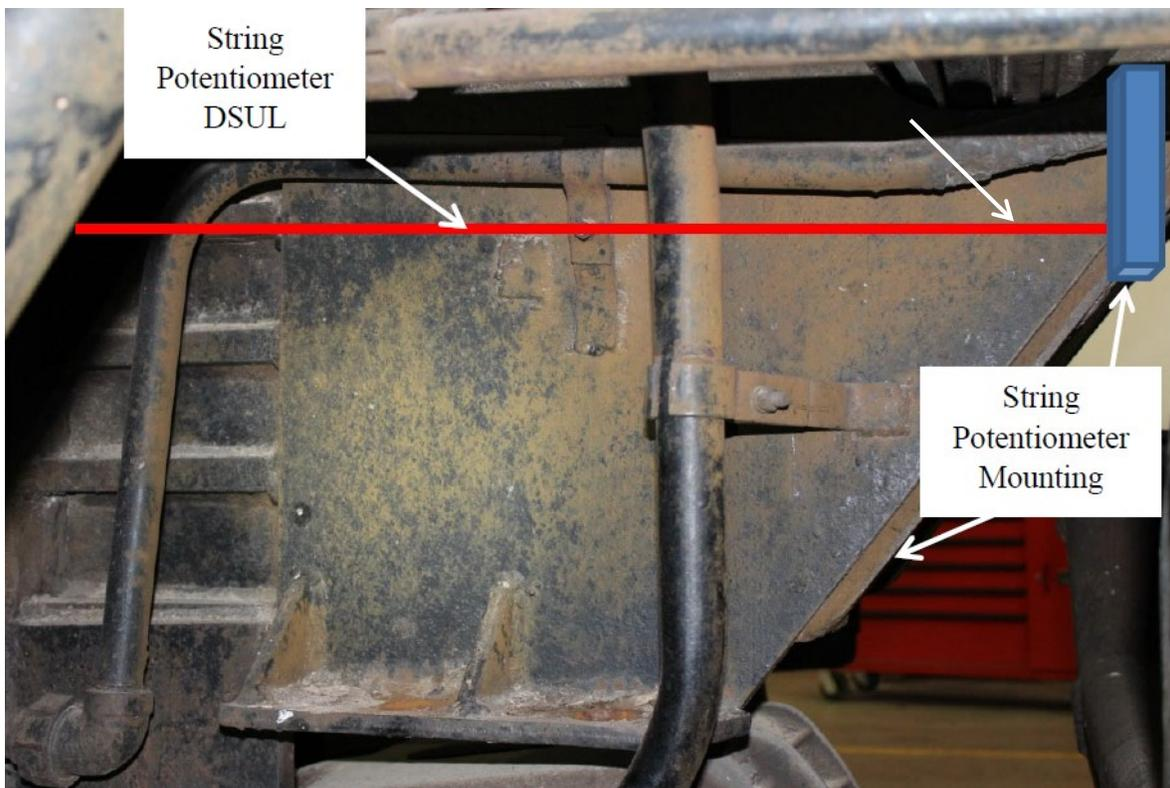
**Figure 20. Stationary Locomotive Underframe String Potentiometer Left**
