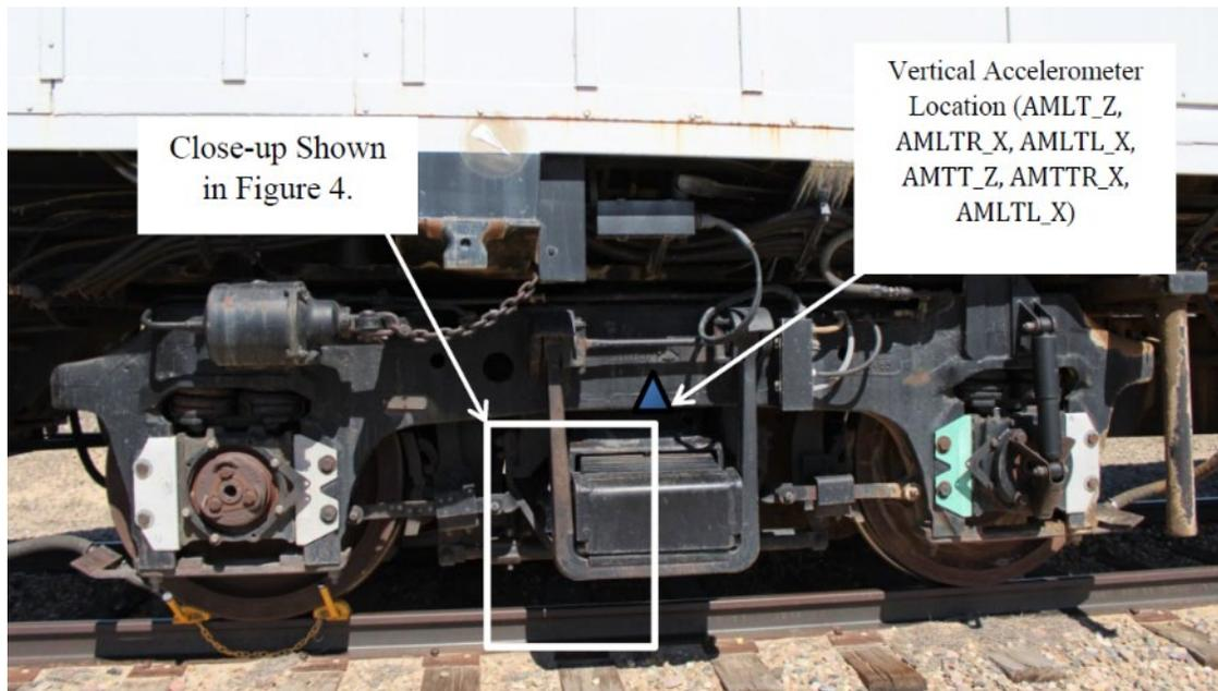
**Figure 4. Locations of Accelerometers on Mobile Locomotive Truck**
