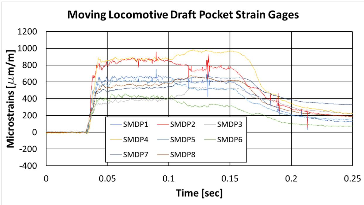
Figure 31. Mobile Locomotive Draft Pocket Strain Results
