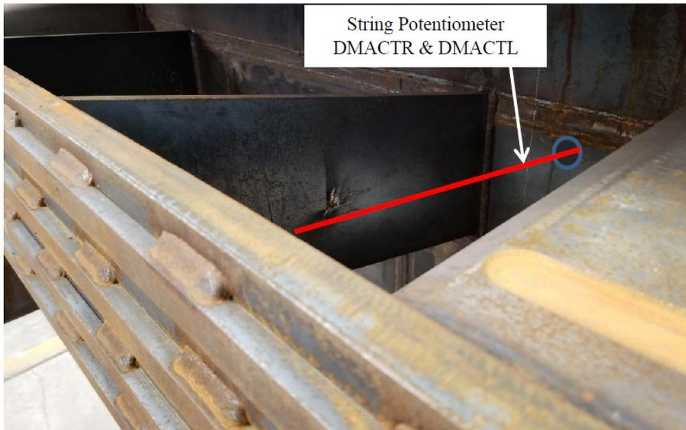
**Figure 7. Mobile Locomotive Top Anti-climber String Potentiometers**
