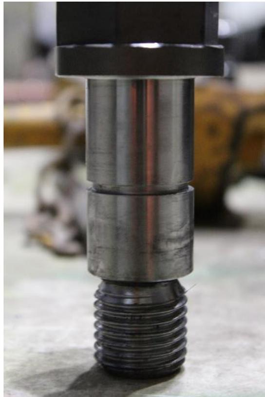
**Figure 43. Intact Shear Bolt After Test**
