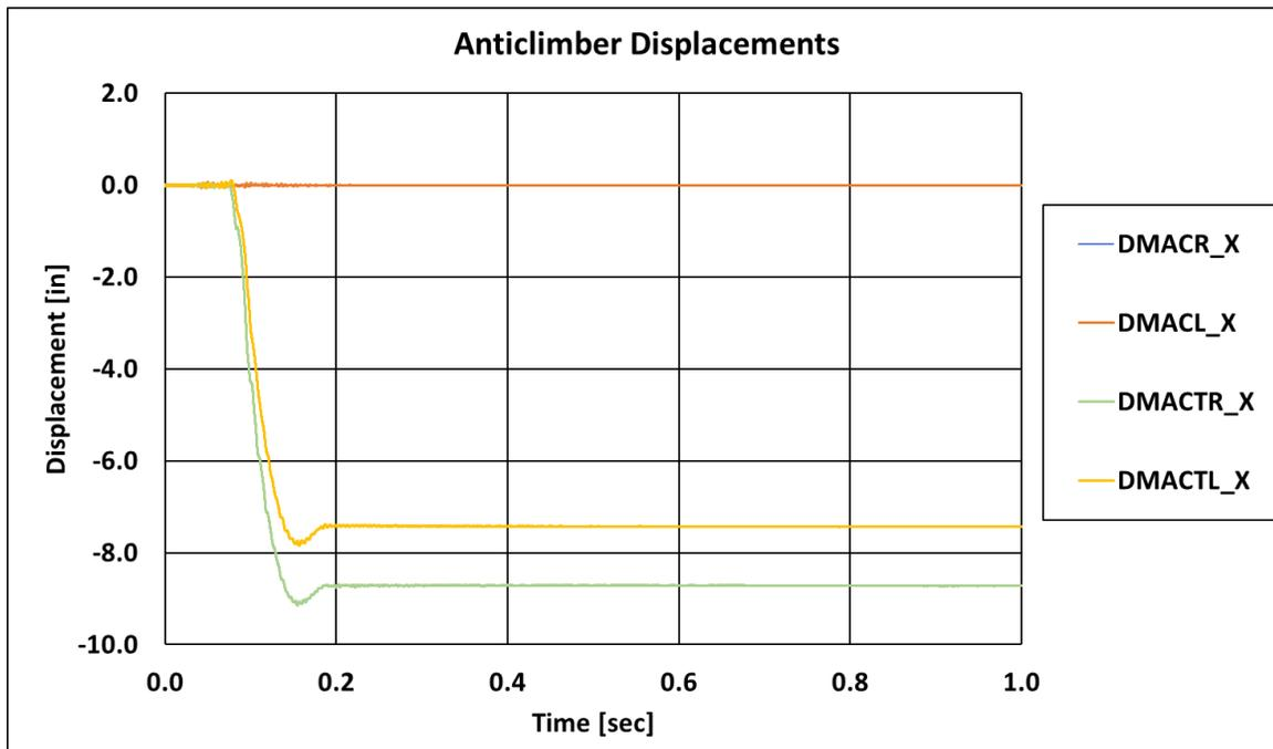
**Figure 28. Anti-climber Displacements**
