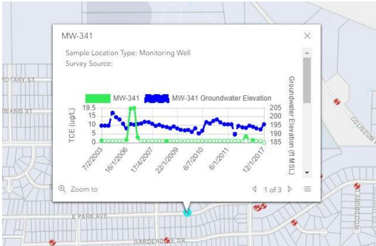
Figure 5. Location pop-up window displays key information including location name, type, and a chart of TCE and groundwater elevation levels.
