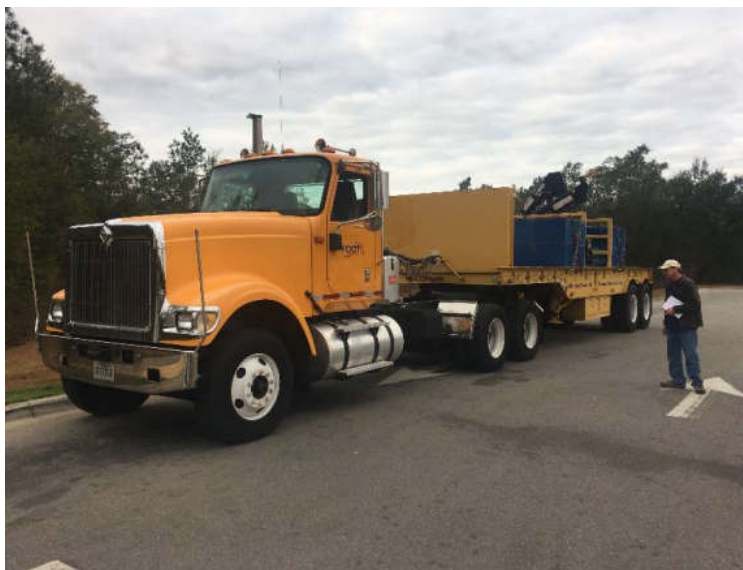
Figure 14 – One of Two Calibration Trucks Used in Florida (Moses, 2019).
