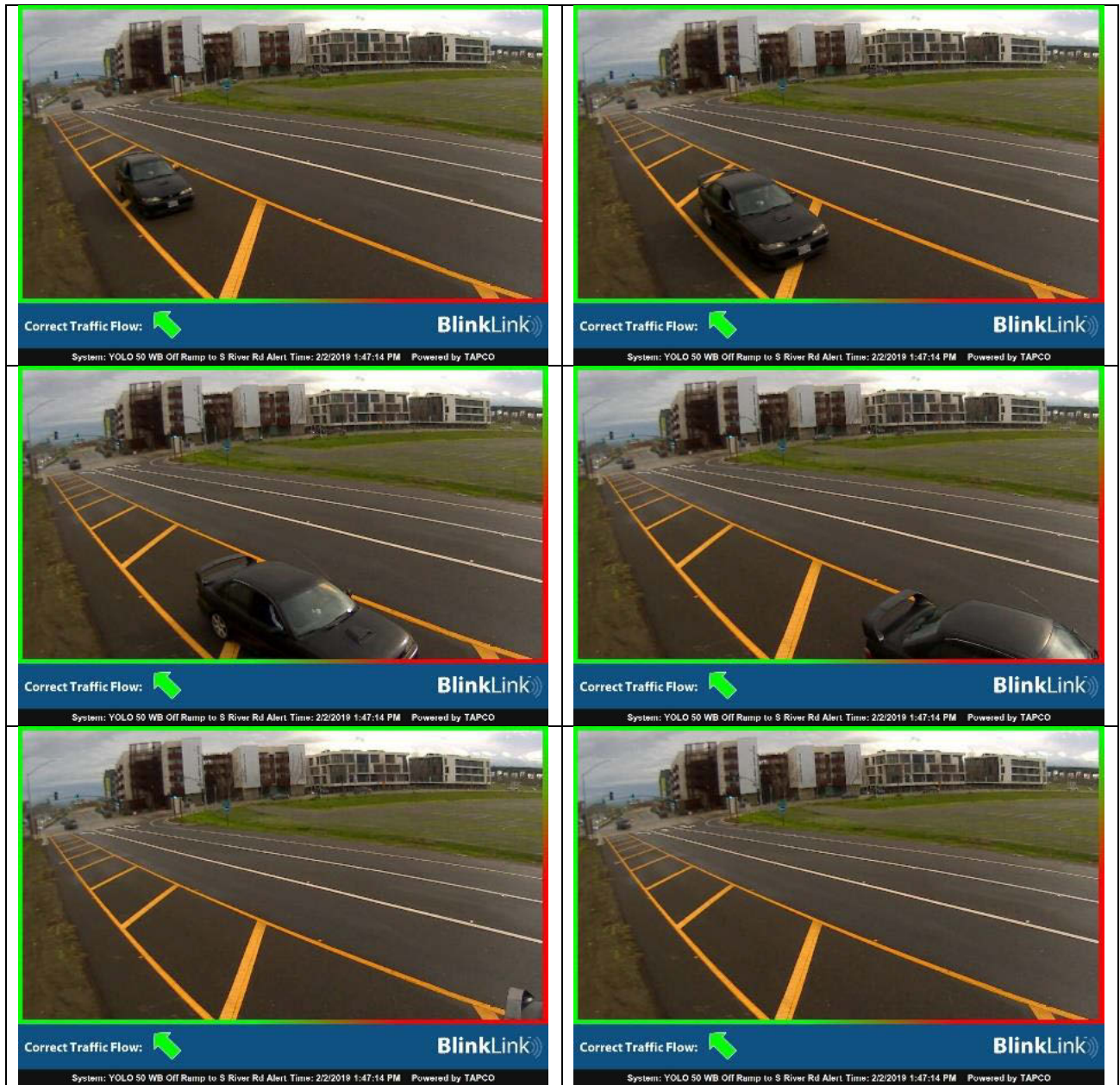
Figure 4.44: Photos (images 7 – 12 of 14) provided by TAPCO system for a typical WWD event. TAPCO provides 14-16 photos for a WWD event. Courtesy of TAPCO.
