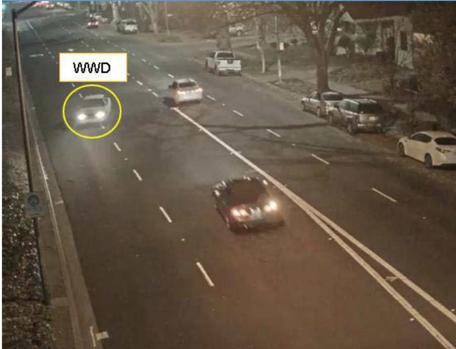
Figure 4.16: Wrong-way driver (circled in yellow) entering the exit ramp at WB US 50 at 10 th Street. The driver continued onto the exit ramp despite at least five cars passing in the other (correct) direction.
