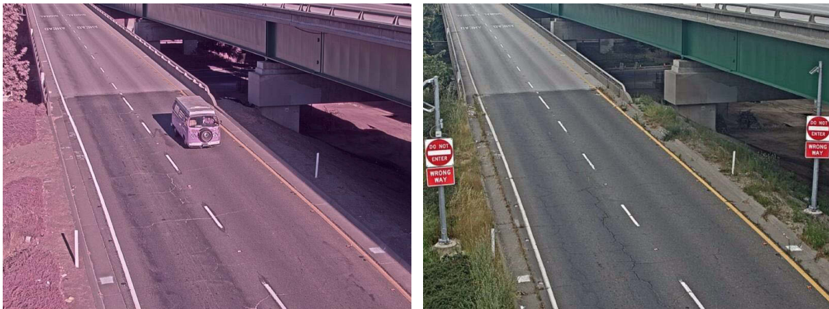
Figure 3.8: Illustration of the IR filter failure. The left image was taken before the camera replacement. The right image was taken after the camera replacement.
