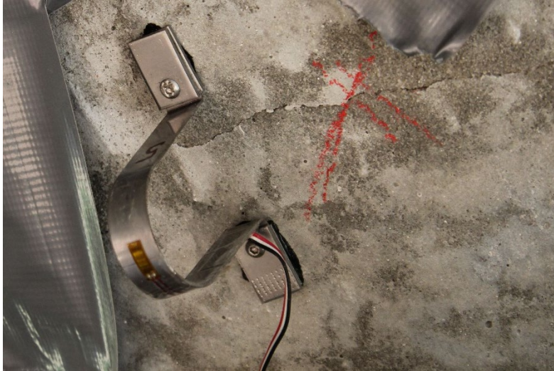
Figure 5.11. PI gauge attached on interior panel 2 to measure crack opening displacement
