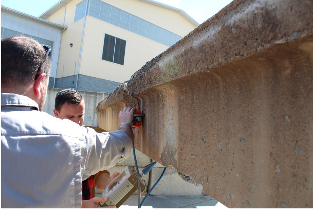
Figure 3.22. Shane Boone demonstrating GPR hardware on concrete double-tee girder
