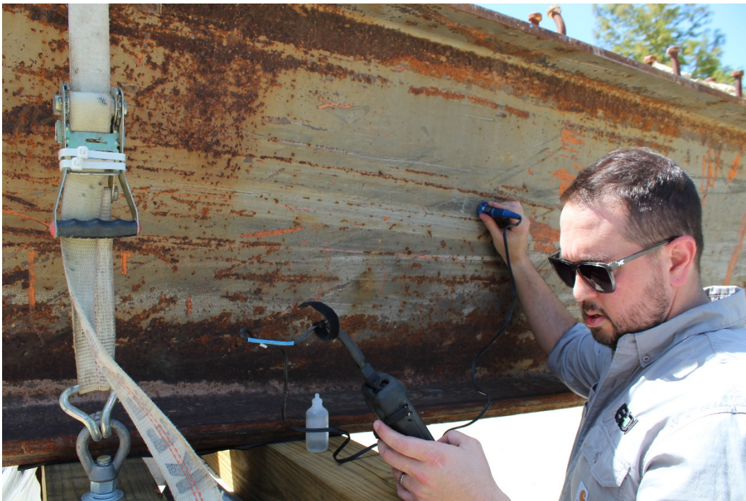
Figure 3.24. Demonstration of ultrasonic thickness gauge on steel beam.
