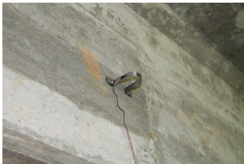
Figure 5.7. PI gauge attached on interior girder 3 to measure crack opening displacement
