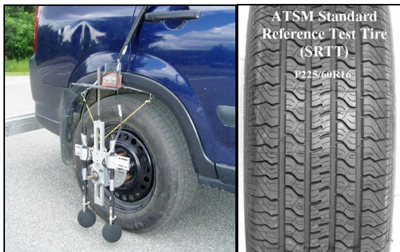
Figure 9. OBSI dual probe system and the SRTT.
