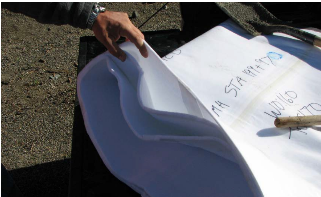
Figure 12. Closeup of the nonimpregnated polyester liner.
