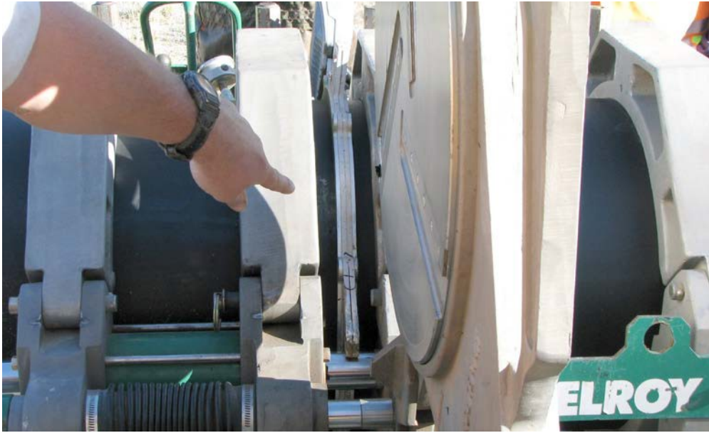
Figure 5. View of the preheated iron during the fusion process.
