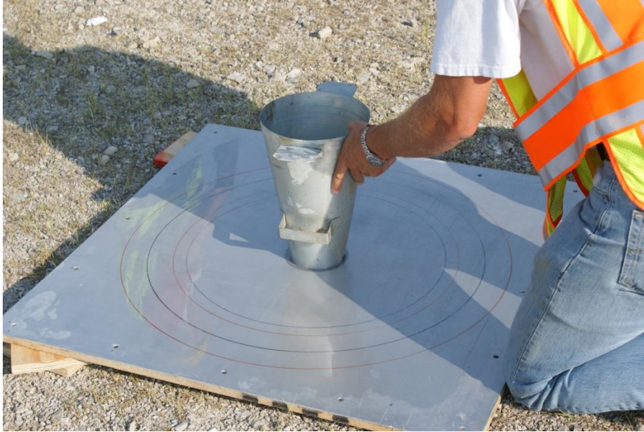
Figure 6. Modified slump test.
