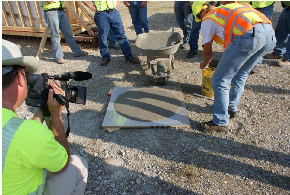
Figure 7. Slump test results from self-consolidating concrete.
