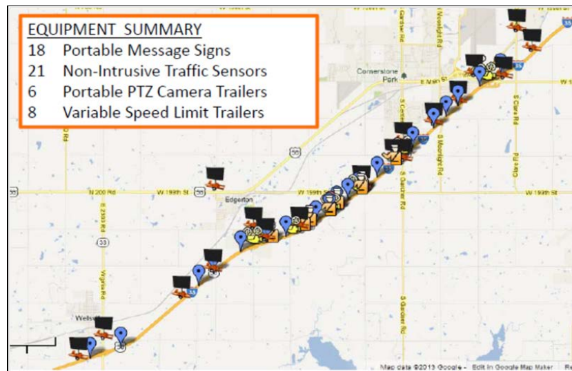
Figure 4. Map. Placement of data collection and message boards along the project (courtesy: KDOT).
