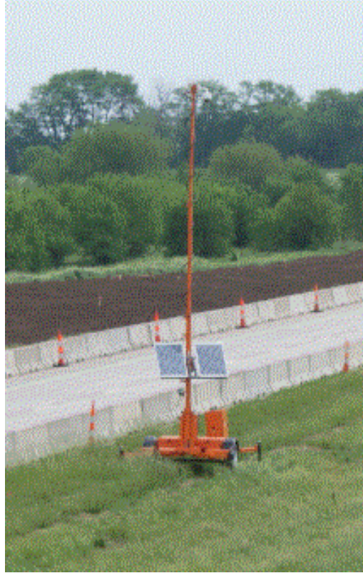
Figure 5. Photo. CCTV trailer.
