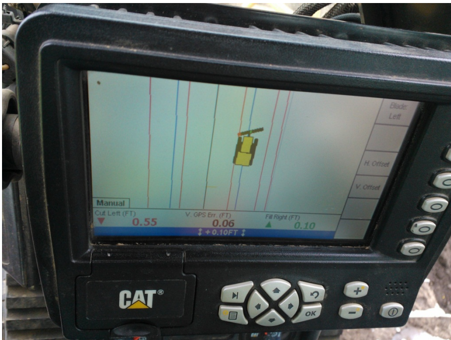
Figure 6. Photo. Screen showing the alignment of the bulldozer.
