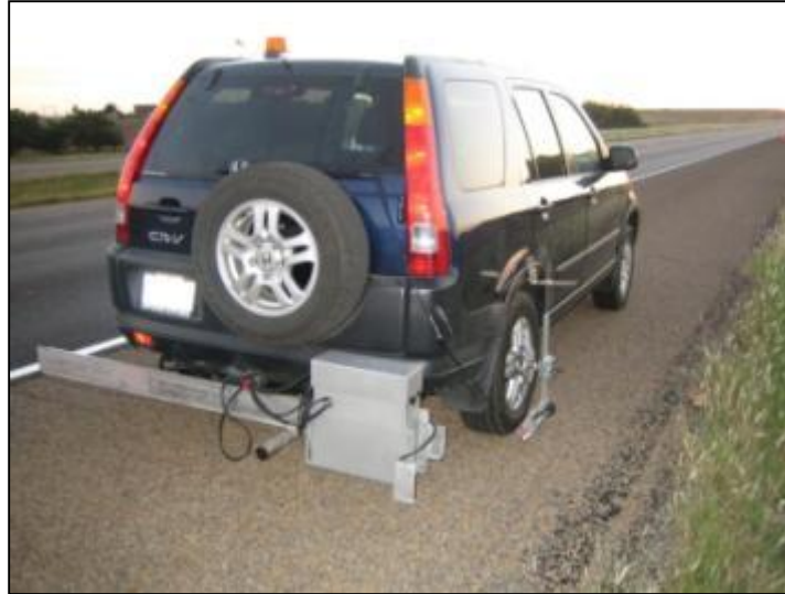
Figure 15. Photo. High-speed inertial profiler mounted behind the test vehicle.
