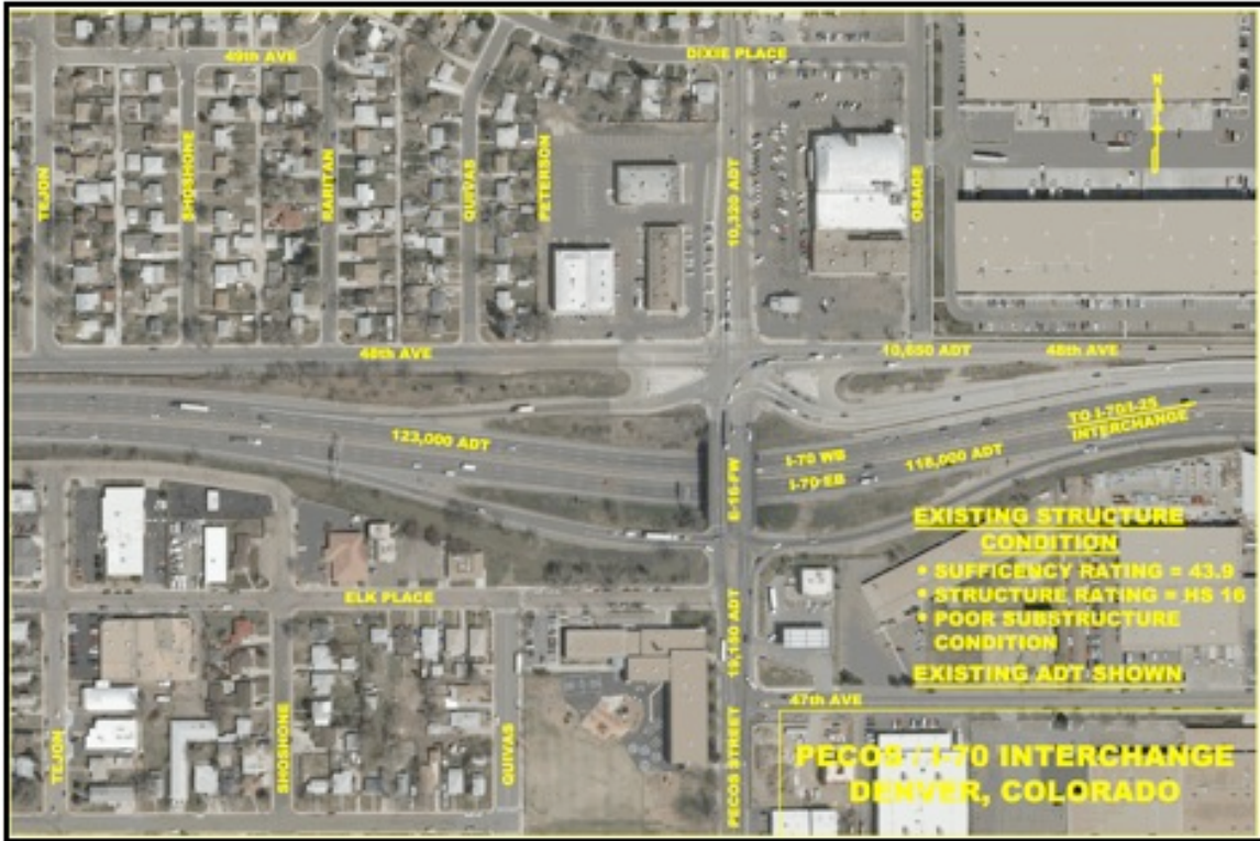
Figure 2. Map. Pecos Street interchange with street layout and traffic information (courtesy: Colorado DOT).
