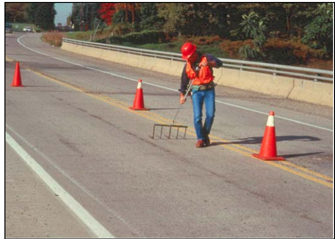
Figure 2.2.28: Inspector Using a Chain Drag
