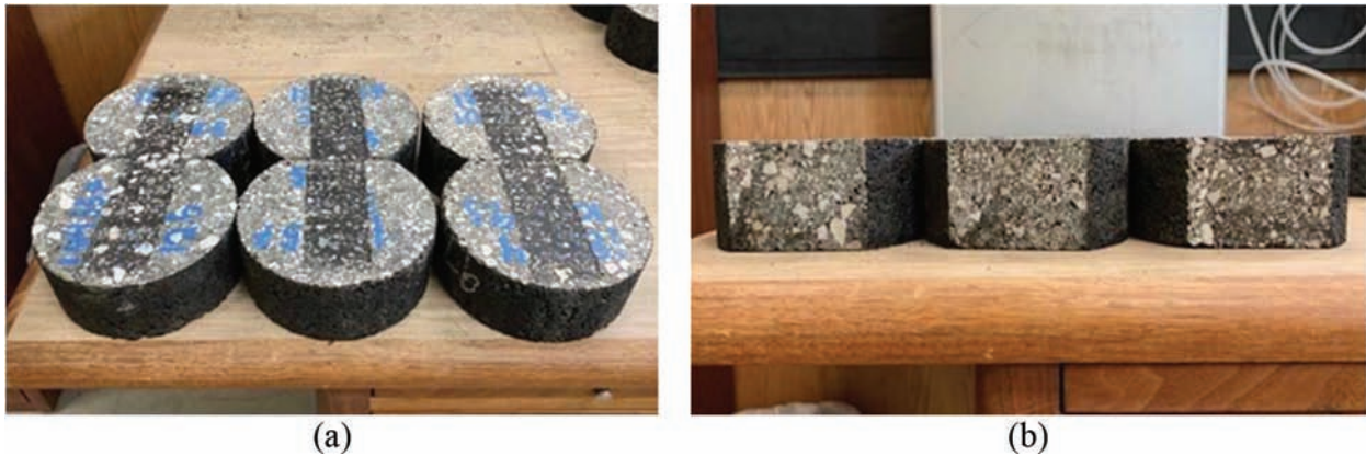
Figure 5.2 Laboratory-compacted specimens after Hamburg test completion: (a) top view (b) side view.
