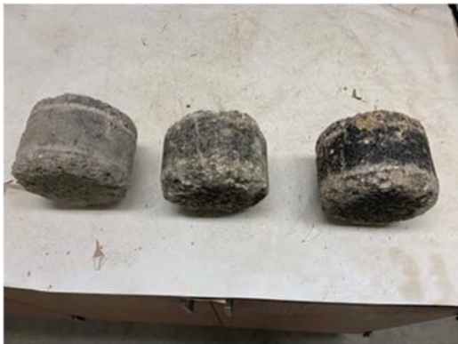
Figure 2.5 Cantabro specimens after testing.
