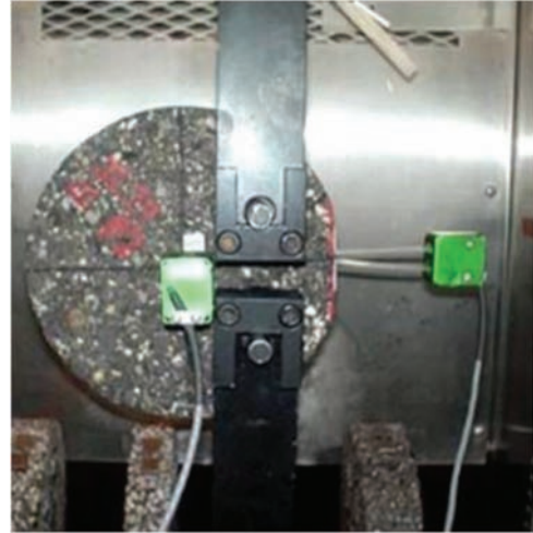
Figure 2.3 DCT setup (Butlar Bill, 2017).
