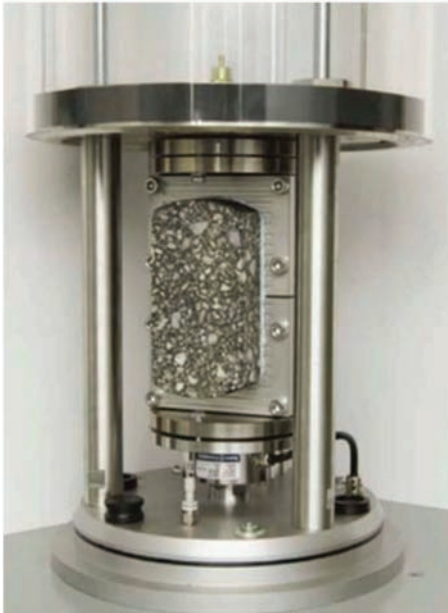
Figure 2.2 Texas overlay test setup. (Controls Group)
