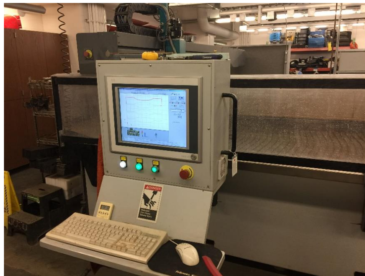
a) Water-jet control system
