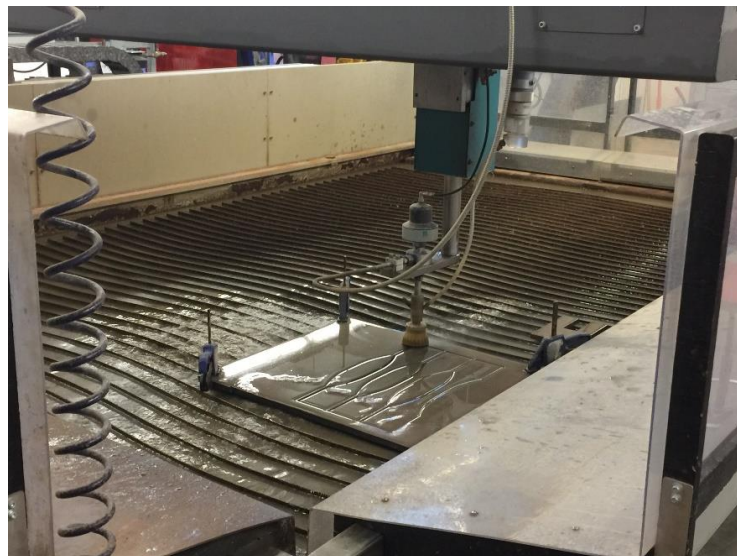
b) Coupon sample cutting
