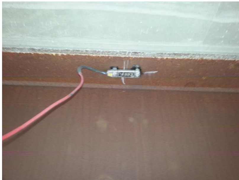
b) Strain gauge setup on A709 steel girder
