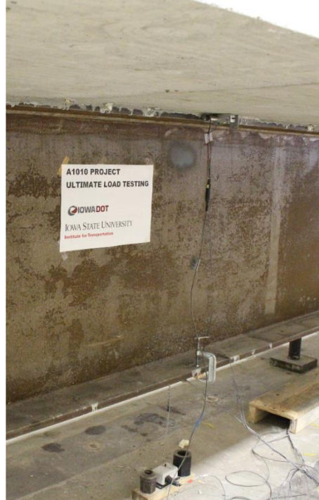
c) LVDT and DCDT at S2 (mid-span)
