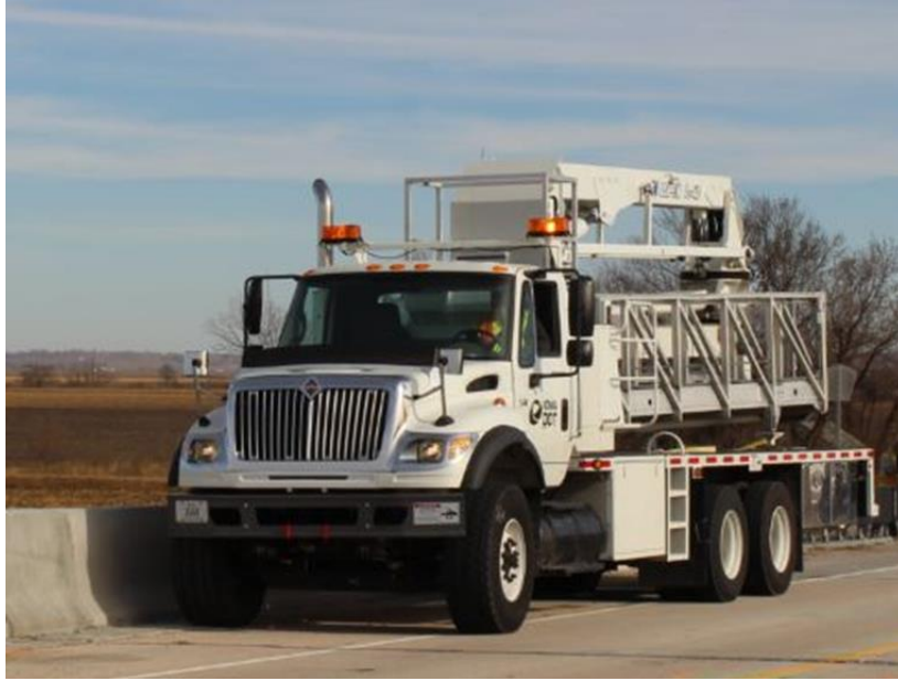
Figure 40. Iowa DOT Salix Bridge load testing truck
