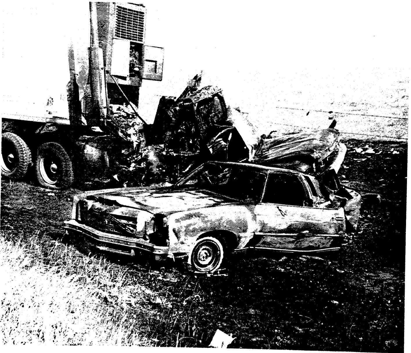
TRUCK OVERRODE REAR OF CAR - CHAIN TYPE COLLISION
