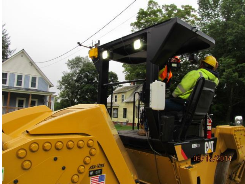
Figure 2. Photo. Paving roller mounted with IC equipment. (courtesy: Vermont Agency of Transportation)
