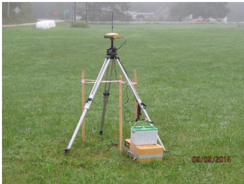
Figure 11. Photo. GPS base station set up over control point. (courtesy: Vermont Agency of Transportation)
