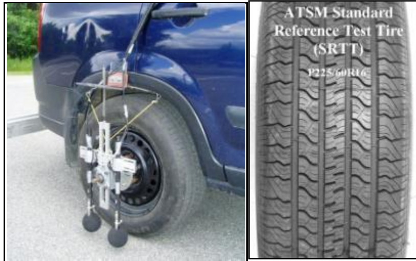
Figure 61. OBSI dual probe system and the SRTT.
