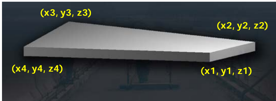
Figure 25. Warped slab geometry in Super-Slab ® design.
