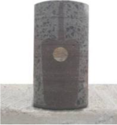
Figure 24. Verification of dowel grout consolidation (cores taken after installation).
