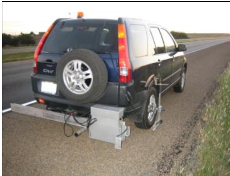
Figure 63. High-speed inertial profiler mounted behind the test vehicle.
