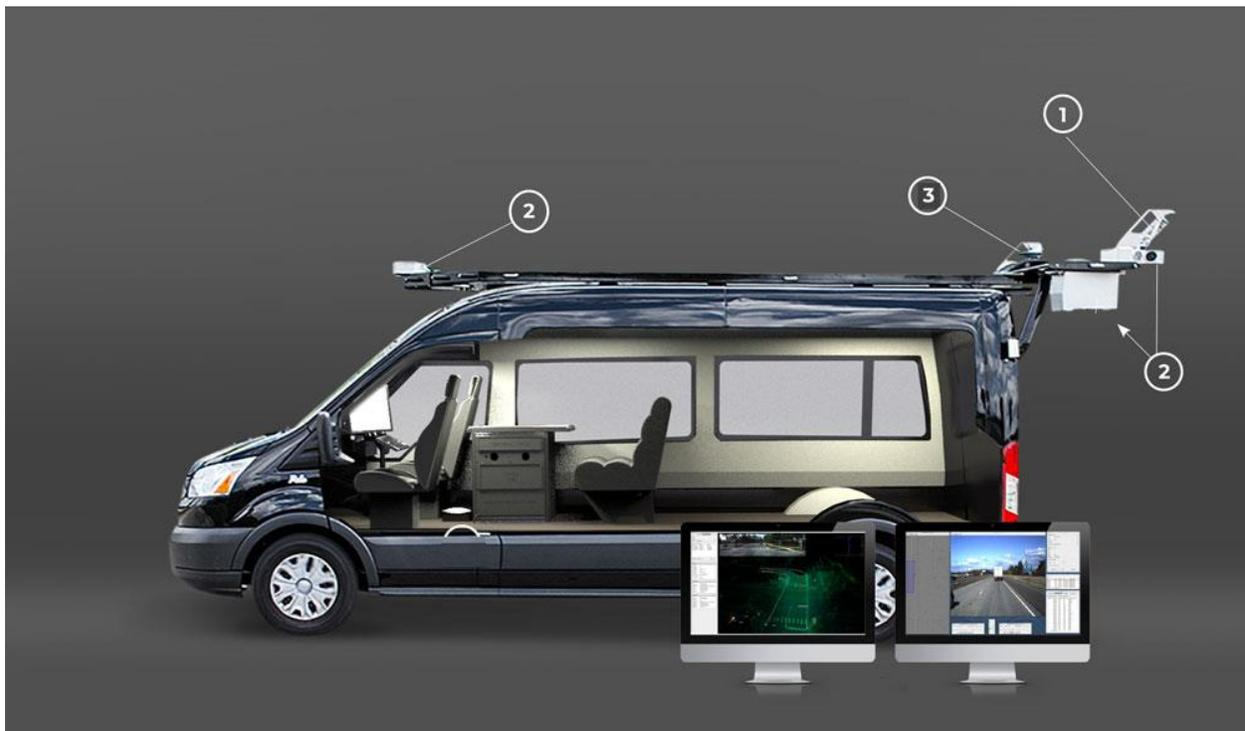
**Figure 2.** The basic components of mobile LiDAR system: 1) dual Velodyne HDL-32 LiDAR sensors, 2) nine 8.9 MP cameras, 3) position orientation system, including GNSS, Inertial Measurement Unit (IMU) and optical Distance Measurement Instrument (DMI). (Modified from Mandli Communications, Inc)
