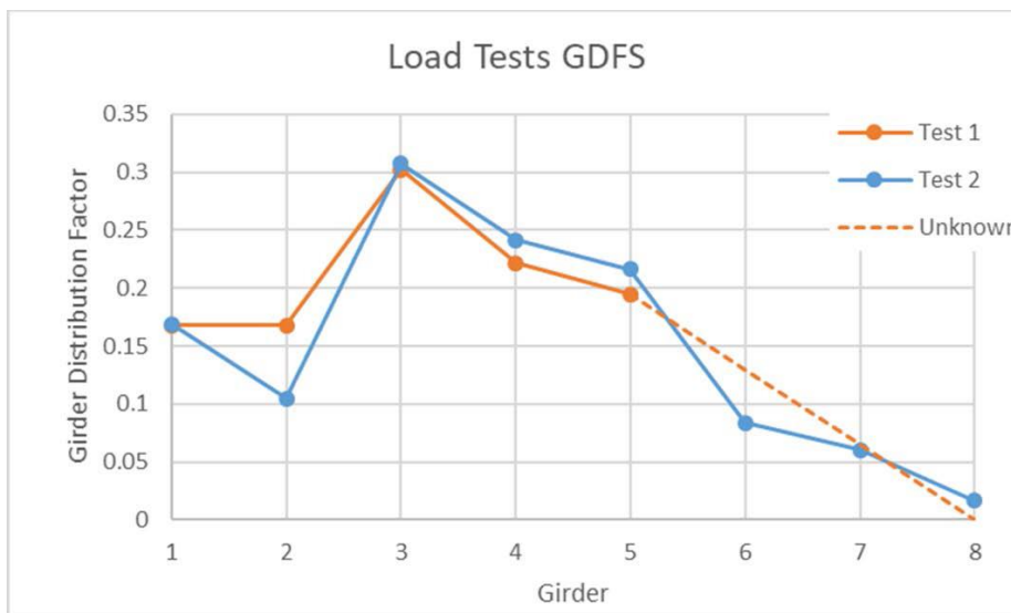
Figure 79. Moment-Fraction GDF Comparison between Tests 1 and 2 for the Critical Interior Girder Load Path
