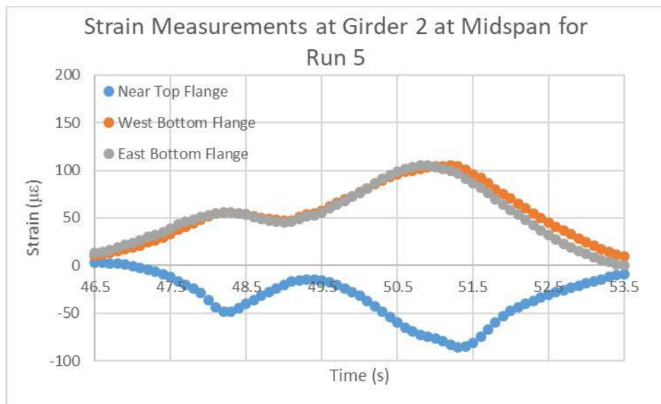
Figure 75. Example Noncomposite Strain Measurements
