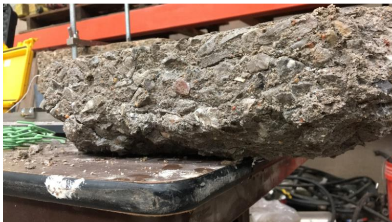
Figure 5-8. Control Mix Specimen at 304 Freeze/Thaw Cycles
