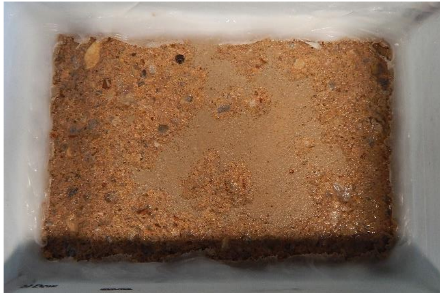
Figure 6-22. 60 Percent Fly Ash Plus 100 Percent RCA After 10 Cycles
