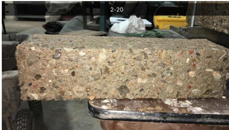
Figure 5-10. Mix 2-20 Specimen at 304 Freeze/Thaw Cycles
