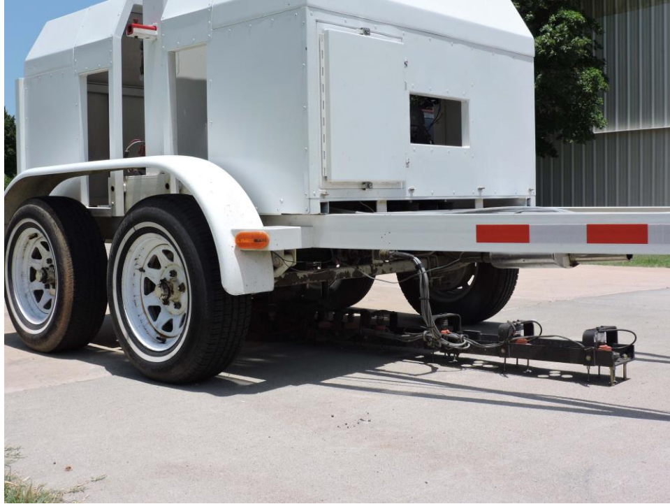
Figure 10-16. FWD Testing of Pavement Panels
