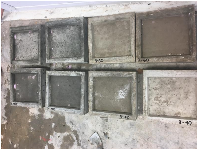
Figure 5-5. Salt Scaling Specimens Air Curing
