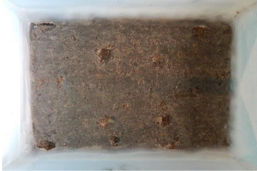
Figure 6-17. 50 Percent RCA Specimen After 50 Cycles
