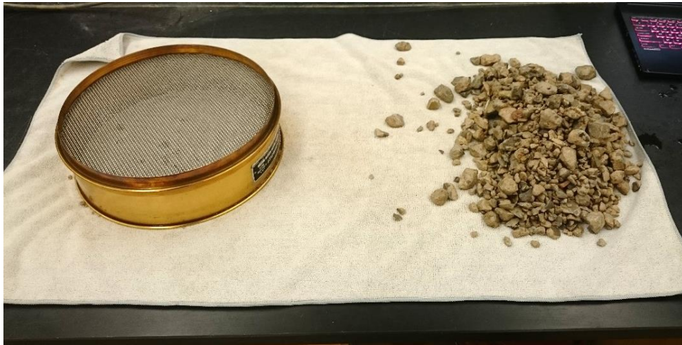
Figure 7-2. Aggregate Preparation for Moisture Measurements
