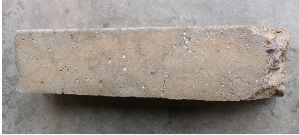
Figure 9-9. Mix 3-40 Specimen at 304 Freeze/Thaw Cycles
