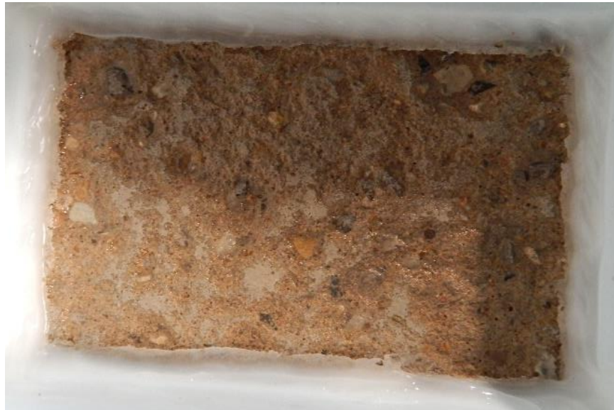
Figure 6-16. 25 Percent RCA Specimen After 15 Cycles
