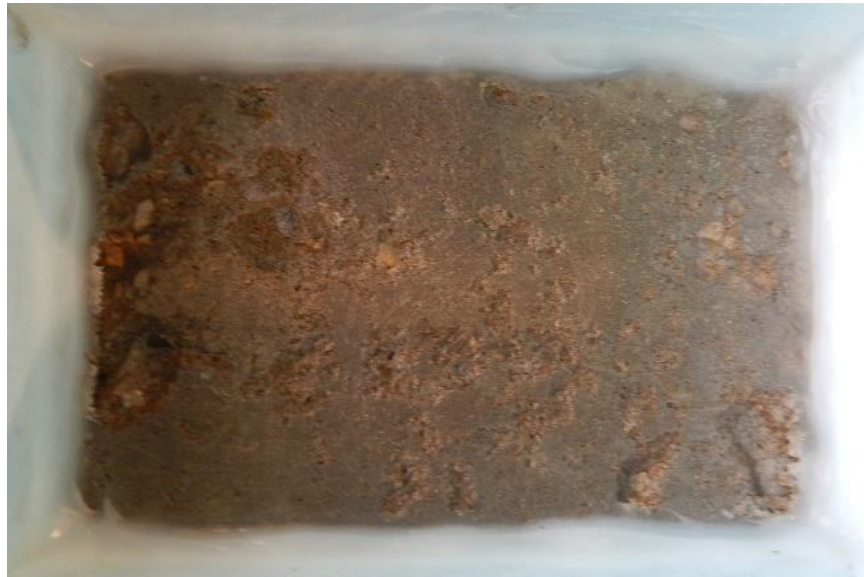
Figure 6-20. 20 Percent Fly Ash Plus 100 Percent RCA After 50 Cycles
