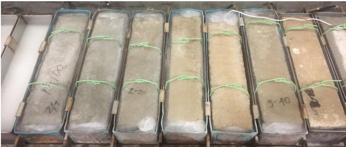
Figure 5-1. Freeze/Thaw Specimens within Test Chamber
