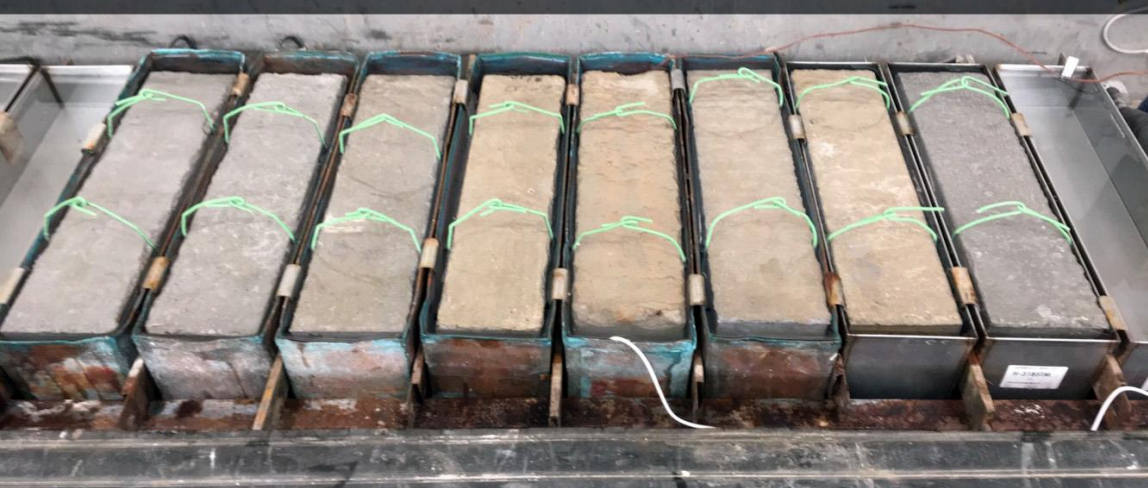
Figure 9-1. Freeze/Thaw Specimens within Test Chamber
