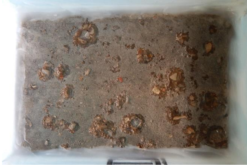
Figure 6-19. 100 Percent RCA Specimen After 50 Cycles
