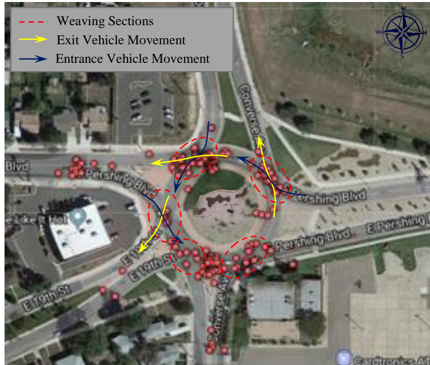
Figure 6.3 Crash Locations within the Cheyenne 2-lane roundabout from 2014 to 2018 (Source: Google Fusion)
