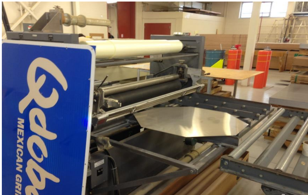
Figure 100. Sign About to be applied with Reflective EC Material.
