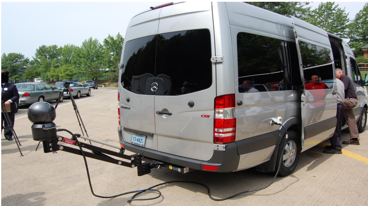
Figure 61. Photo. An Infrared Inspection System with an External Infrared Camera (Federal Highway Administration, 2003).
