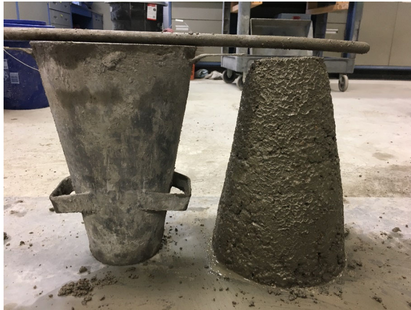
Figure 3.6. Slump test setup
