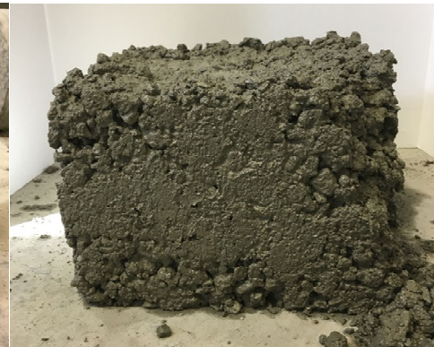
d) 4a-failed edge quality
