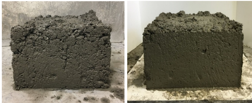
c) Example of poor performance d) Example of good performance
