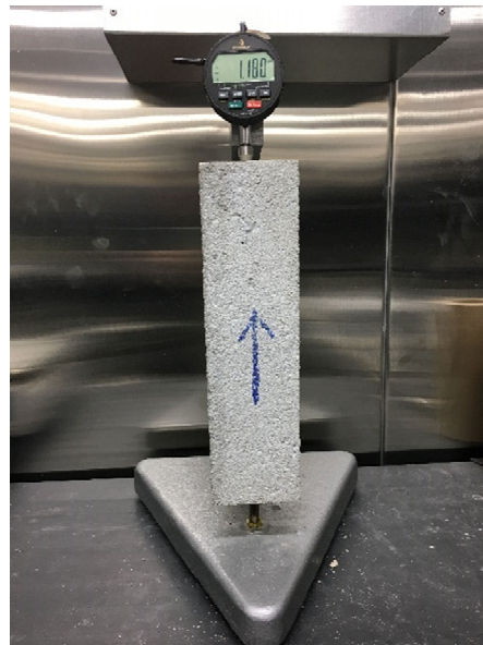
Figure 3.17. Length comparator used for shrinkage measurement
