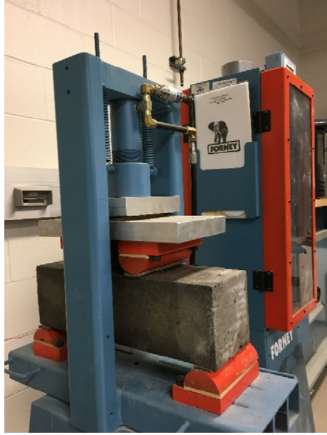
Figure 3.13. Flexural strength test setup
