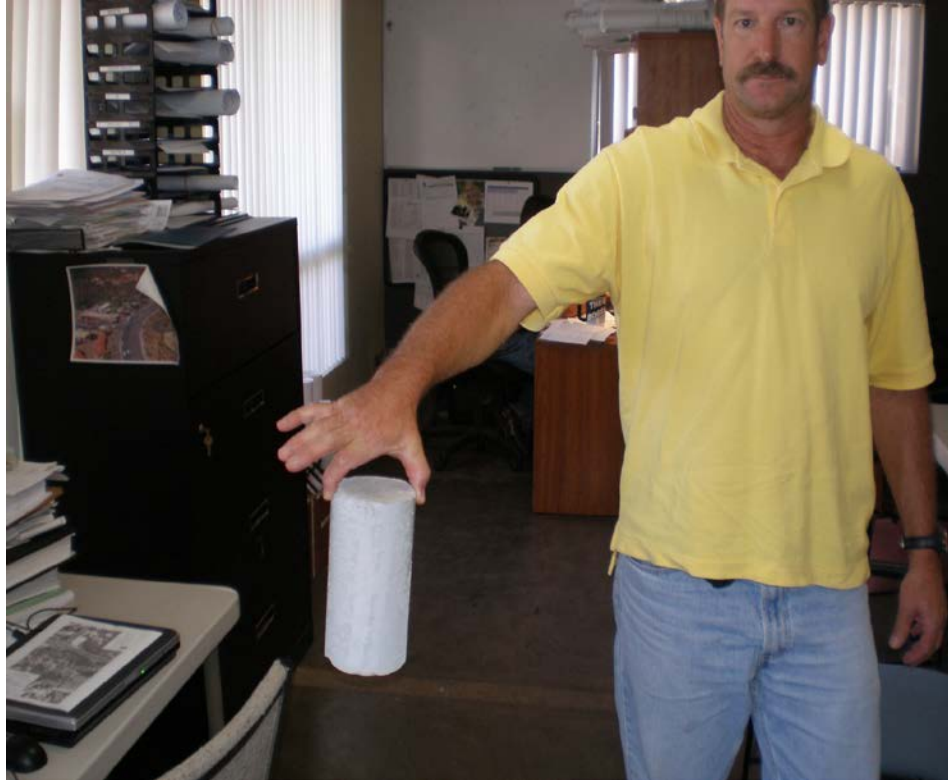
Figure 13. Demonstrating the lightness of a 4x8-in foamed concrete cylinder.
