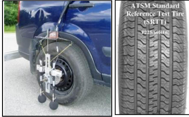
Figure 22. OBSI dual probe system and the SRTT.
