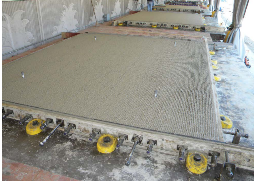
Figure 11. Longitudinally textured surface of a freshly made panel.
