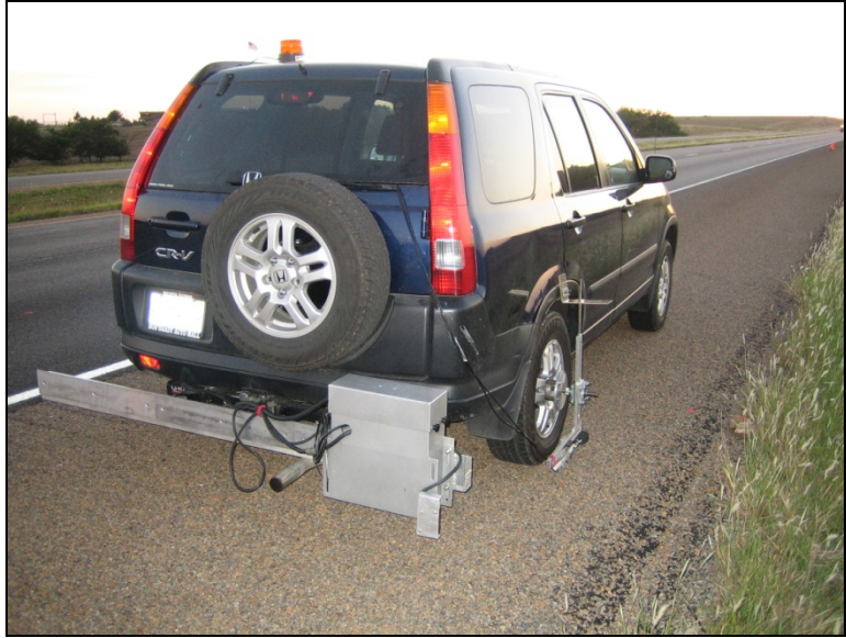
Figure 21. Laser profiler mounted behind the test vehicle.
