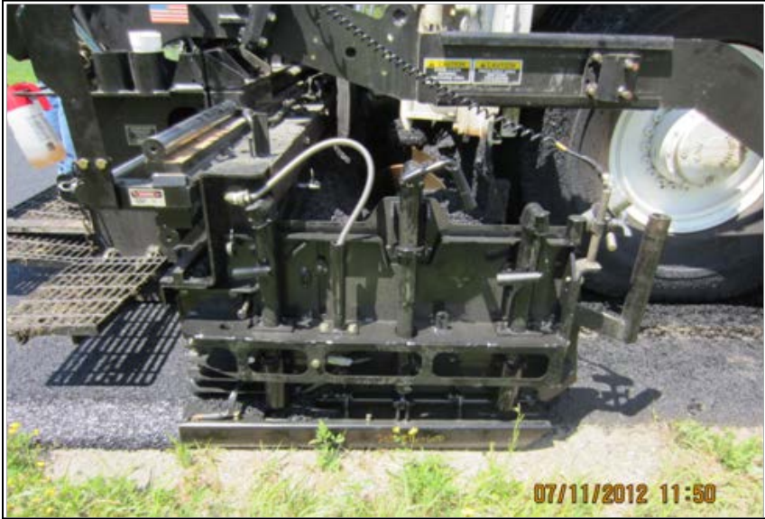
Figure 40. Closeup of Carlson Safety Edge device attached to the end plate of the screed.
