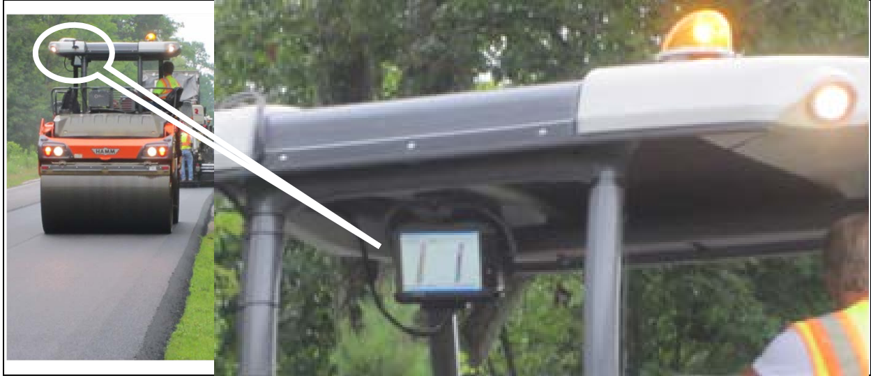
Figure 18. Display screen on the HAMM IC roller for monitoring coverage and other parameters.
