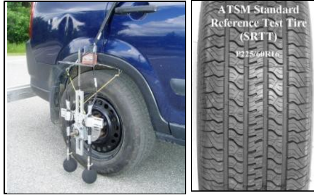
Figure 19. OBSI dual probe system and the SRTT.
