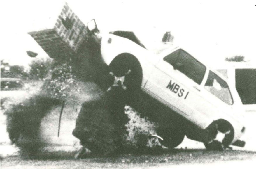
Figure 6. Mailbox Stand and Vehicle Impact Test MBS-1
