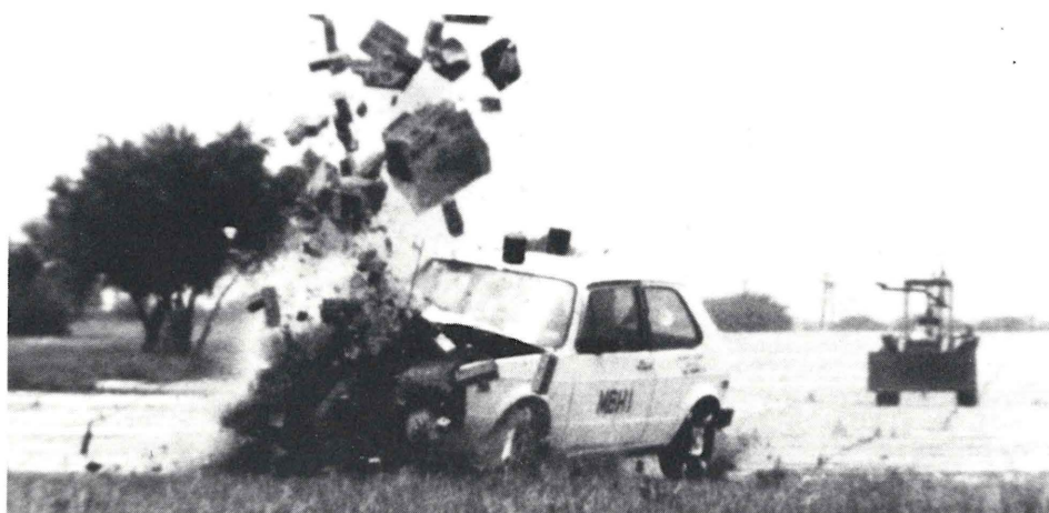
Figure 3. Mailbox Stand and Vehicle Impact Test MBH-1
