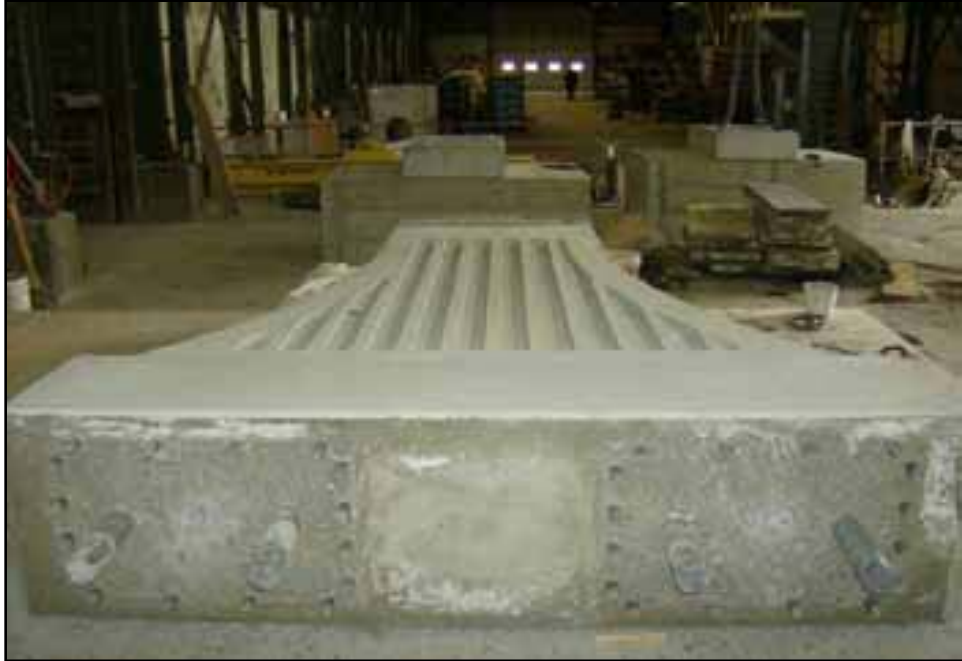
Figure 7. Manufactured precast pier unit.
