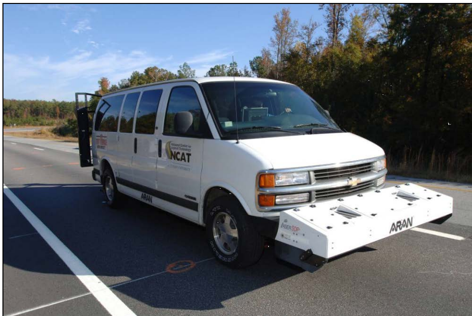
Figure 19. Auburn University ARAN van. (Source: NCAT)
