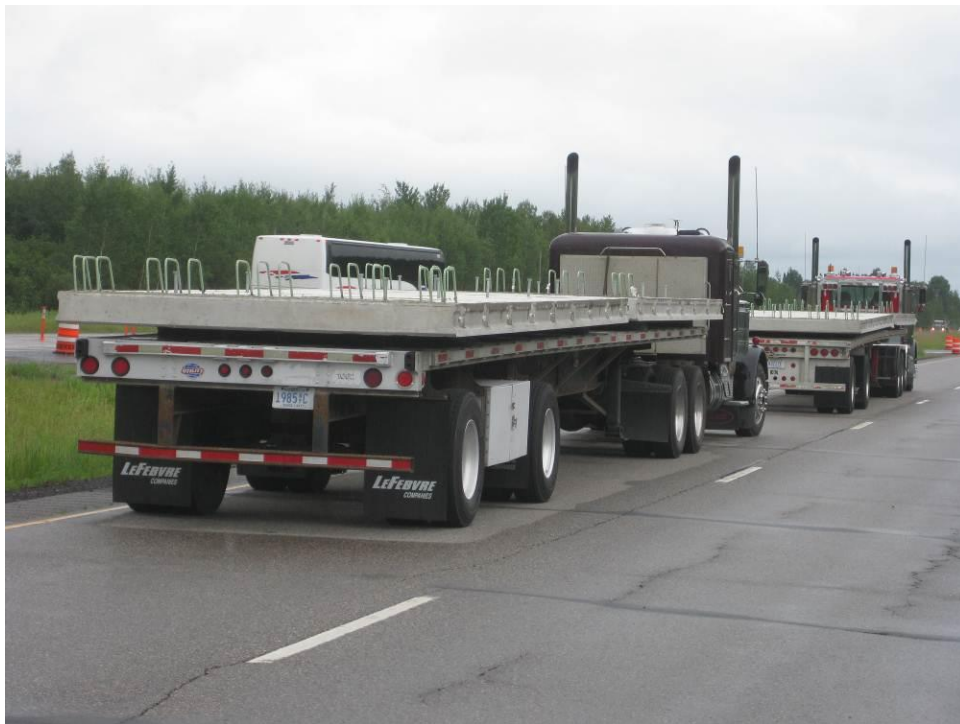
Figure 20. Transportation of precast deck panels on flatbed trucks to bridge site.
