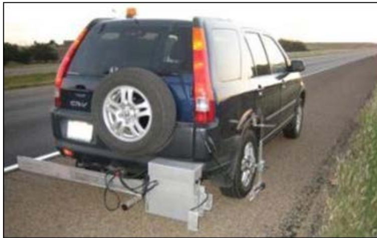
Figure 25. High-speed inertial profiler mounted behind the test vehicle.
