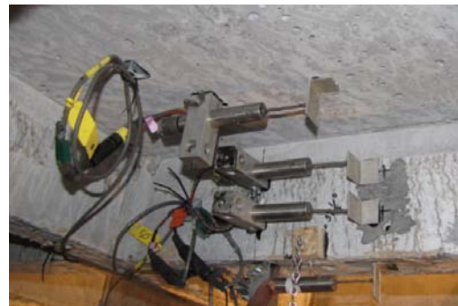
c) LVDT attached to a transverse rib
