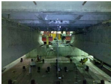
b) String potentiometer configuration
